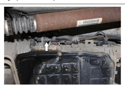
6. To remove connector, push red tab (1) downwards. Then, press the black tab (2) which will allow the white handle (3) to be rotated downwards, releasing the connector from the transmission.
