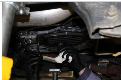
35. Place the supplied gasket on the transmission pan. Hold pan below transmission and install attaching screws. Torque the pan screws to 105 in/lbs.
