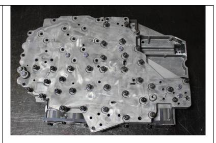
27. Re-install solenoid pack onto valve body. Be sure to properly align the pin on the solenoid pack with the slot on the valve body. Due to the alignment dowels, the valve body may need to be wiggled down into position. Install solenoid pack attaching screws. Install remaining Torx screws to fasten the solenoid pack to the valve body.
