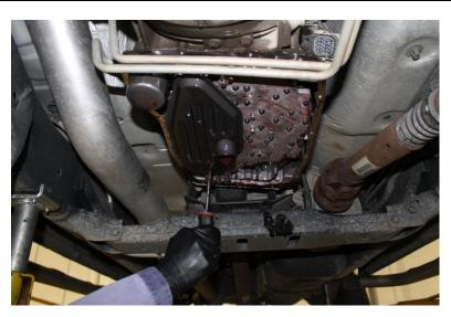
11. Remove the six 8mm bolts securing the valve body to the transmission. Drain valve body of fluid. To remove valve body from transmission, wiggle it while pulling downwards to work the electrical connector through the case.
