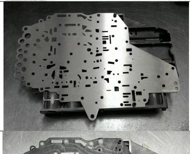
25. Install the second BD valve body gasket part number 1600186-2 on the separator plate, lining it up with the dowels.
