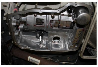
33. Torque the valve body attaching bolts to 105 in/lbs.
