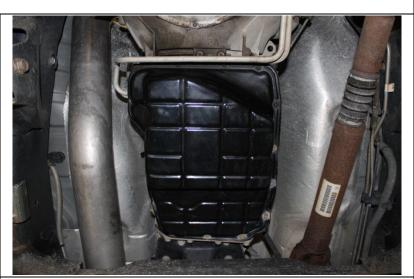
Tap pan with a mallet to break the silicone gasket seal. Allow fluid to drain. Remove last screw and drain remainder of fluid.
