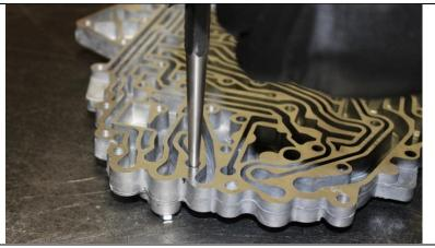
19. Drill hole with 1/8" drill bit.
