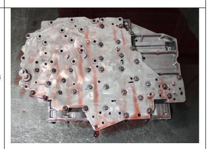
13. Remove fifteen T25 Torx screws securing the solenoid pack to the valve body, remove solenoid pack and place it to the side.
