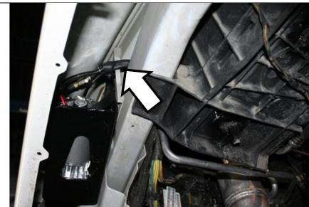
Secure the compressor in place by reinstalling the hood hinge bolt through the compressor bracket. Then install the nut and bolt to hold the front of the bracket.
