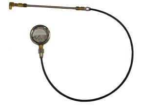
To test the idle pressures, the exhaust brake must be applied at idle. If the engine is cold, the brake will turn on when at idle, otherwise it must be commanded manually.
