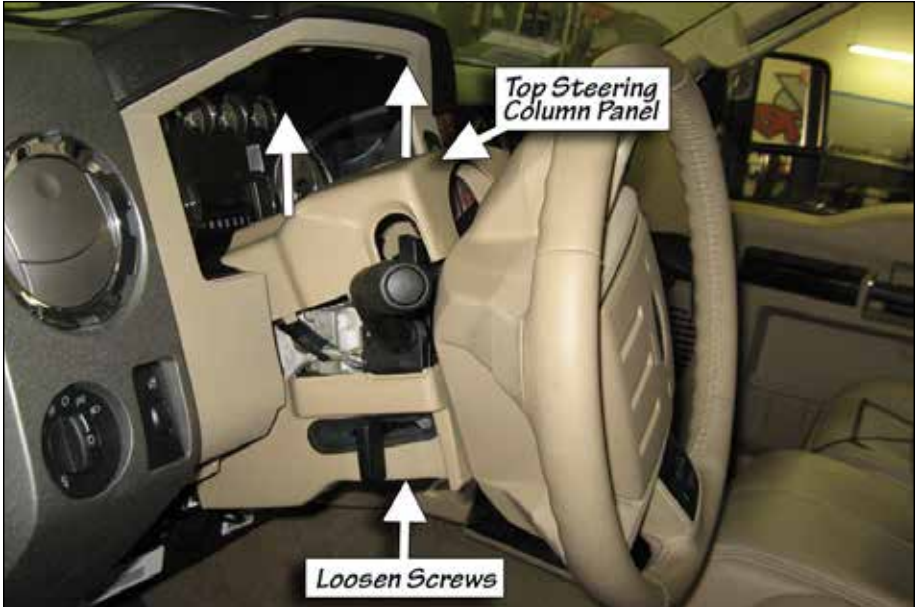
Figure 13 Remove top column panel cover
