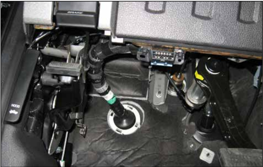
Figure 6: Rubber Grommet on driver side Fire wall
