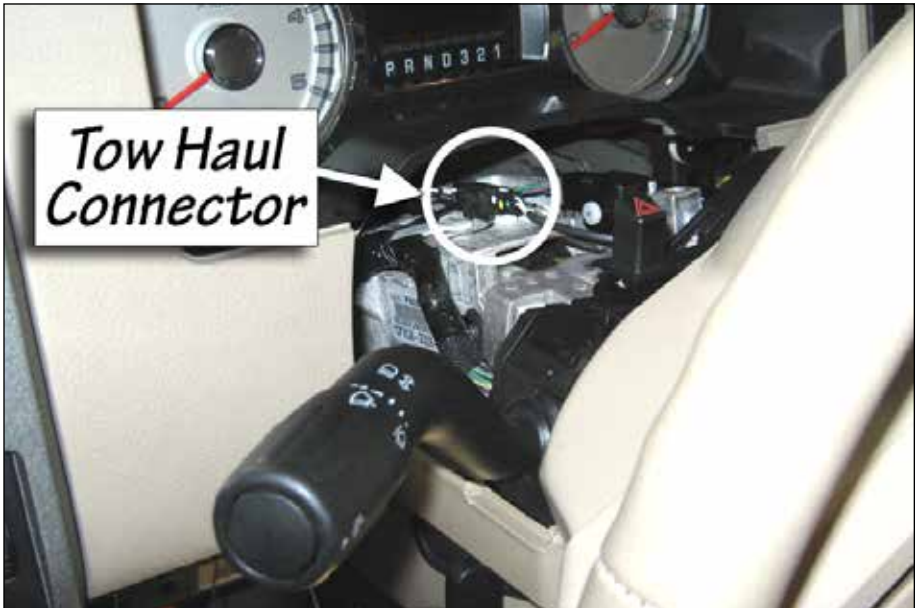
Figure 14 Tow Haul Connector on steering column, under main harness
