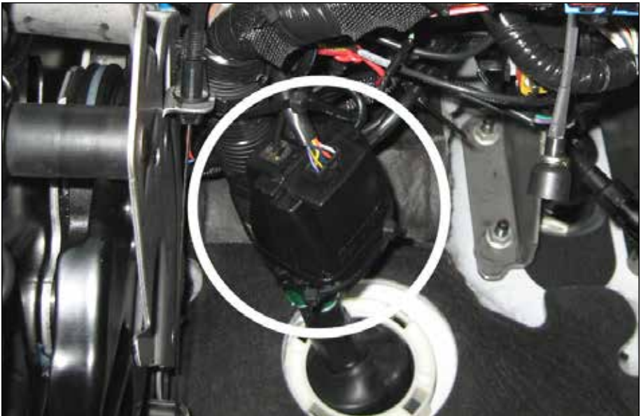
Figure 15 Banks Brake Module mounting location
