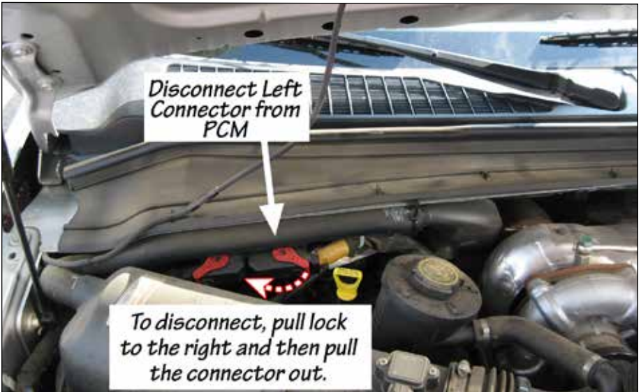
Figure 3: PCM Location on Passenger side.
