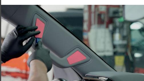
Beware: If you use a screwdriver, it could leave a mark on the soft plastic. A plastic pry tool and/or rag is recommended.
