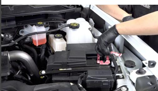
1. Before starting the installation, use your 10mm socket to remove the terminal and disconnect both batteries.
