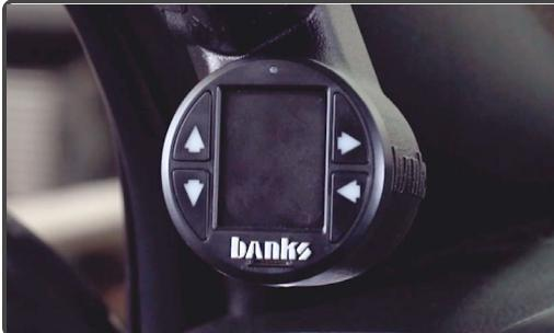
Make sure the Banks logo is aligned correctly. Then reinstall the plastic cap that hides the upper bolt on the pillar.
