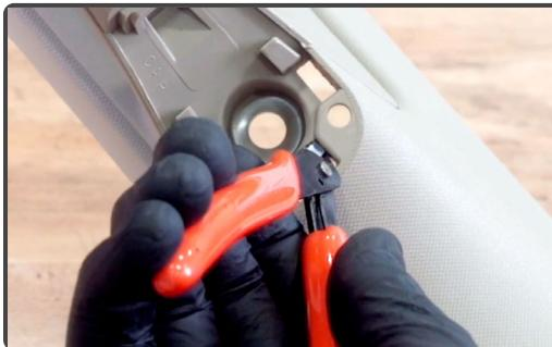
To start, make a single cut here and move to the left side and make an identical cut.
