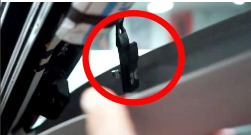
**IMPORTANT NOTE:** Some trucks have an airbag retaining strap connected to the pillar. Please look before pulling it off to see if your truck has one. If it does, slide the strap out of the clip, and then remove the pillar.
