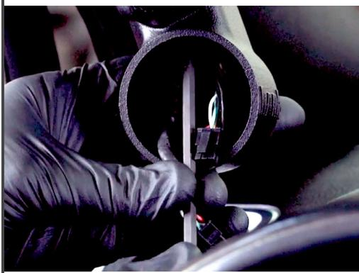
Start threading the bolt by hand and then use the supplied 5mm hex key to finish securing the Stealth Pod in place.
