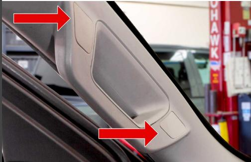
Beware: If you use a screwdriver, it could leave a mark on the soft plastic. A plastic pry tool and/or rag is recommended.
