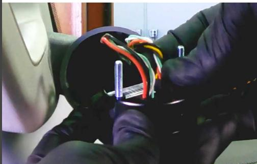
Press the iDash into place, taking care to route the cables back to through the hole and into the pillar as you go.
