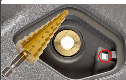
Depending on which Stealth Pod you have, you may need to drill above or below the mounting bolt. Always check which pod you have before drilling.
