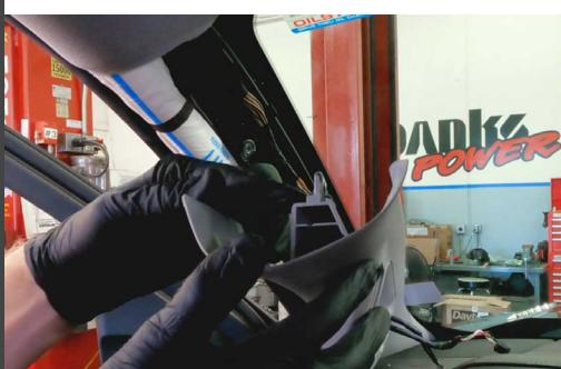
When you're satisfied with the fit, snap the clip on the top back into the truck.
