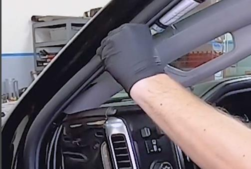
8. Slide the pillar into the dashboard so it fits flush and looks just like the passenger side.
