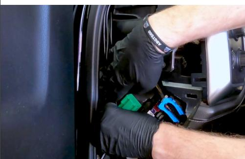
Fish the wires through the metal pillar and down the dash to the fuse box area or out the bottom of the dash, depending on which Banks devices you have.
