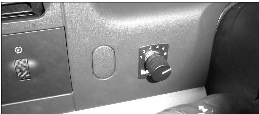
Figure 51: Finished installation of the Power Level Selector Switch on 2005-07 model year vehicles
