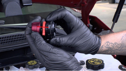
Be sure to line up the tabs before rotating the locking ring.
