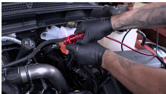
Carefully line up the alignment tab on the starter cable with the Derringer, and fully seat the cable before locking it.
