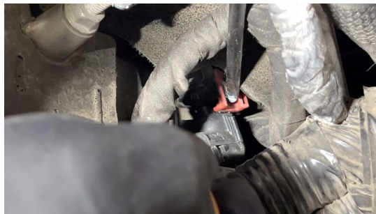
When the red safety lock has been slid back, use a pick or flat-blade screw driver to push the tab like a button.
