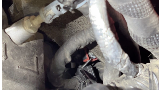
Using a pick tool, lift up the tab slightly.
