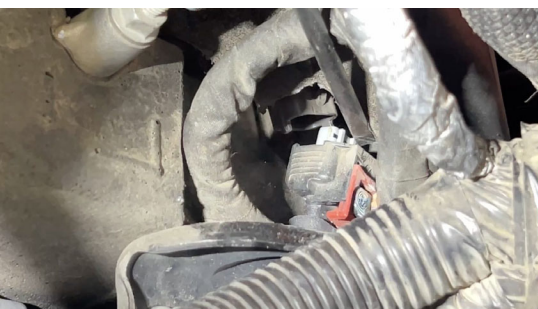
This will release the plug, allowing you to remove it from the injector.
