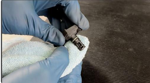
A rag or brush can be used for stuck-on debris.
