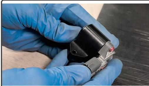
Thread the factory T15 Torx screw by hand, then tighten snugly.
