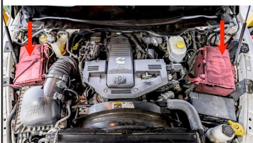
Before unplugging your MAP sensor, it is important to disconnect both batteries and let the ECM discharge for at least 15min.
