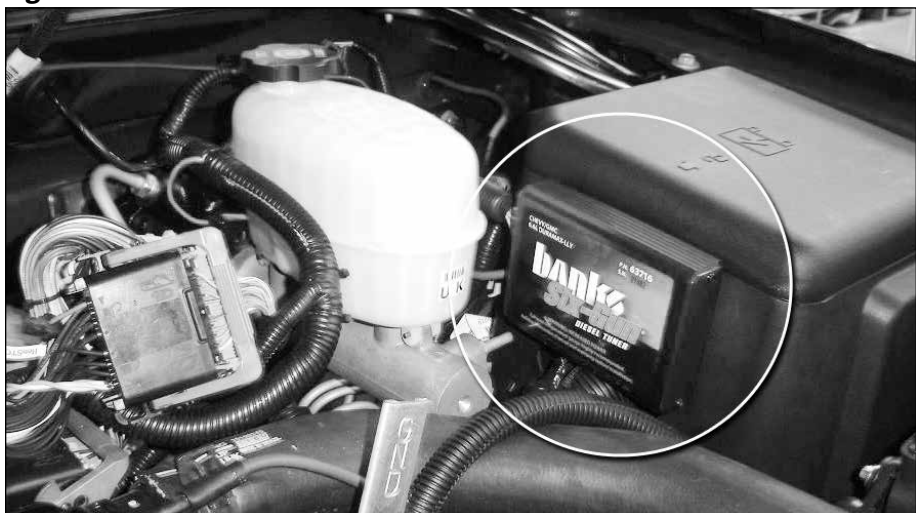
Figure 4 Six-Gun module mounted on fusebox
