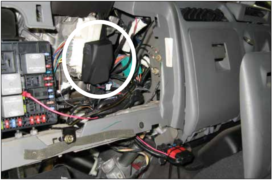
Figure 23 SpeedBrake Module Mounting Location
