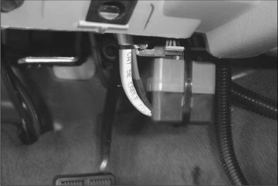
Figure 19 Brake Position Sensor location under dash
