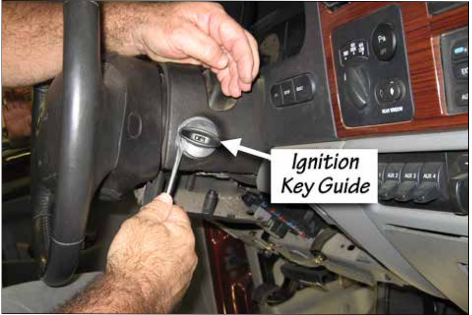
Figure 21 Remove Plastic Ignition Key Guide
