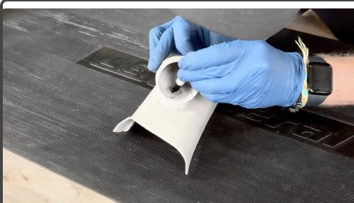
Test fit your stealth pod and mark the center of its cable access hole
