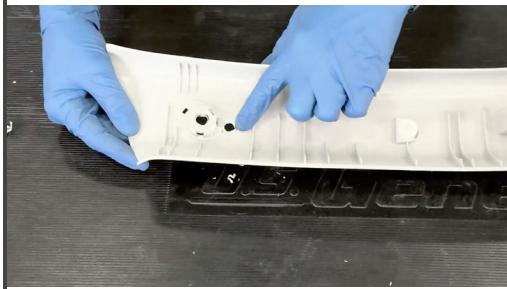
You may need to drill the hole from both sides to remove all the scraps of plastic.
