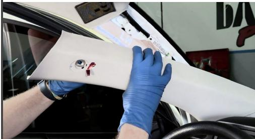
Drape the extra out of the access hole as you snap the pillar back into place.
