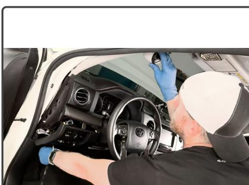
Take up the extra slack as you slide the iDash into place. There should be just enough to pull the iDash back out if needed.
