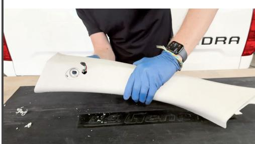
12. Back at the truck, Check how long the end of the OBD-II cable should be. This will be the goal length once you run the small end up your A-Pillar and cable tie any excess.
