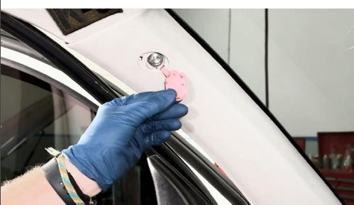
The SRS bolt is a bit tricky to remove using a screwdriver without causing a scratch. Using a pick is recommended.
