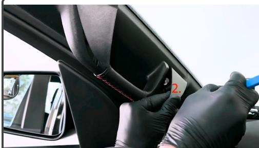
A plastic pry tool is recommended to avoid scratching the plastic surface.
