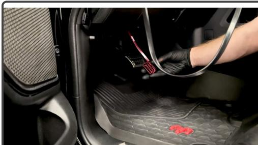
Leave enough slack at the end to plug the cable into the OBD-II port.
