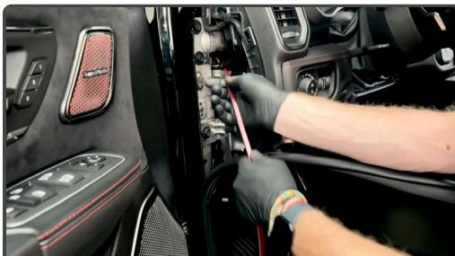
Feed the OBD-II plug through the side access panel.
