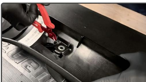
The back side of your hole can be cleaned up by a pair of snips.
