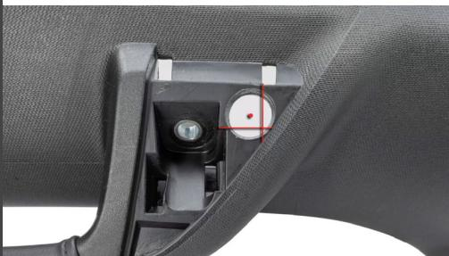
The center of the drill bit will be in-board of the corner you made. That way, the hole will be hidden behind the Stealth Pod.
