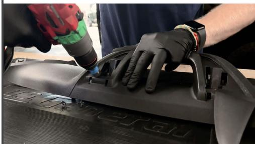
Drill until the 16mm or 18mm step. 16mm for a single cable or 18mm for two.
