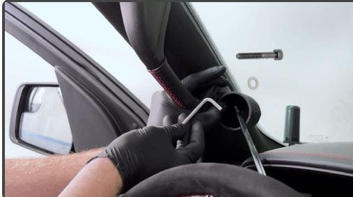
Install the supplied Hex bolt with the included key.
