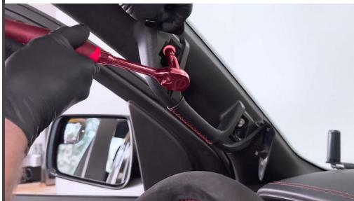
5. With a 10mm socket, remove both bolts.
