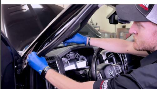
3. Pry the side dashboard cover open to gain access to run cables through.
