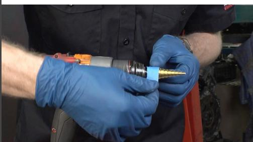
11. Start drilling 90° perpendicular to the spot you marked.
