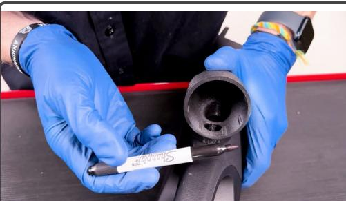
With a marker, place a dot in the center of the cable access hole onto the pillar.
