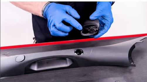
7. Test fit your Stealth Pod to see where you should drill your cable access hole
