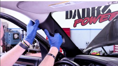
6. With a firm tug, remove the pillar from the vehicle.
