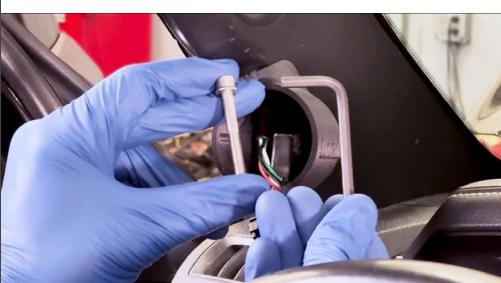
13. Run your cables through your Stealth Pod, and attach it with the supplied bolt and Hex Key.
