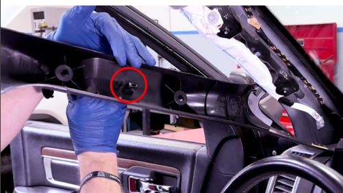
It is being held in by this plastic tab. One firm yank should free it.
