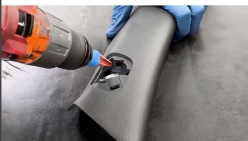
You will need to drill to the 16mm step for a single iDash cable, or to 18mm if you have a PedalMonster.
