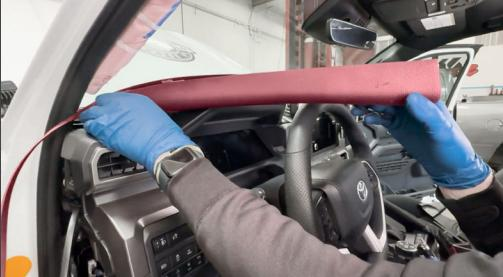
The far end of the A-Pillar as a tab that helps guide and center the pillar to the dashboard. Be sure this tab slides into place or the pillar won't fit.
