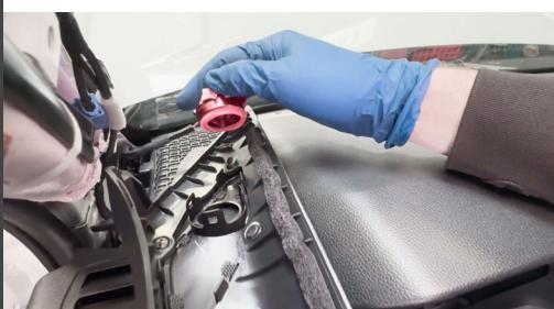
18. Run your cable through the cable access hole you drilled earlier.
