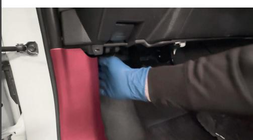
It is being held in by this plastic clip, just pull the cover loose for now to provide access to run your OBD-II cable later.
