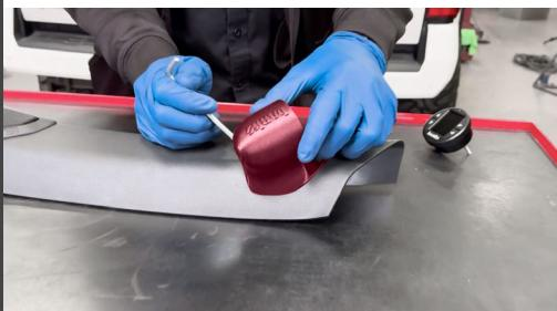
12. Test fit your Stealth Pod to see where you should drill your cable access hole.
