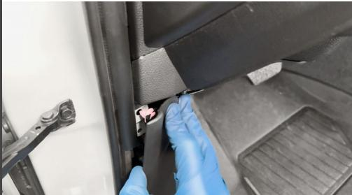
Re-attach the lower finger nut that holds the kick panel in place.
