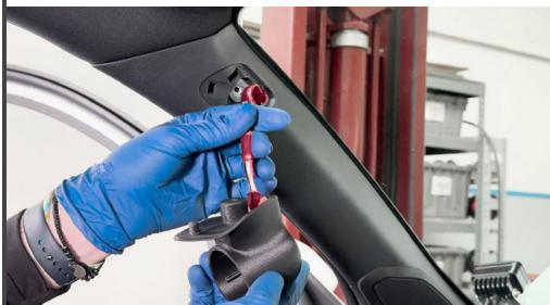
Tighten to 8-10 in-lbs. Due to the design of this Stealth Pod, over-tightening the bolt can cause a failure in the plastic.
