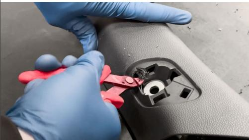
A pair of flush cutters can be used to clean up any excess.
