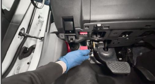
24. With the included zip ties, tidy up the excess wires and secure them together so they won't rattle around when driving.
