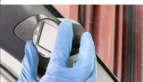
Pull the excess wiring back through the A-Pillar, leave just enough free so you can pull the iDash out if needed.
