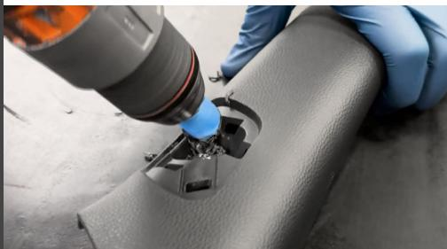
Drilling again from behind can help clear the cut plastic from the pillar.
