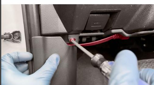
27. Snap the lower kick panel back in making sure the plastic tab lines back up.
