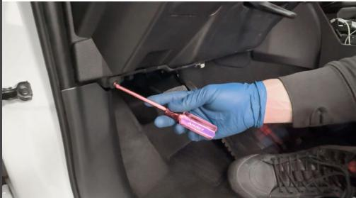
9. With both the screw and nut removed, firmly pull the kick panel towards the rear of the truck to pop it free.
