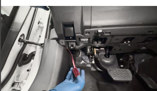
16. Fish the other end of the OBD-II cable up the side and drape the cable(s) over your dashboard for now.
