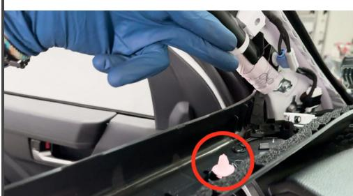
5. If your truck has a tweeter speaker, carefully remove it by lifting the plastic tabs around the speaker.
