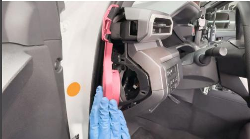
26. Secure the single Philips screw you removed, taking care to route the OBD-II Cable cleanly through the gap.
