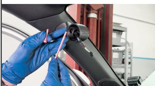
Please hand-tighten until the pod is snug against the factory pillar. Do not tighten beyond this point.
