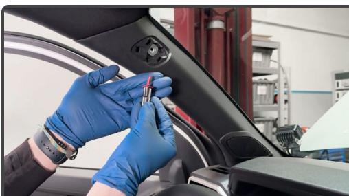
4. With two hands, reach around the plastic A-Pillar trim piece, and pull firmly to the right, towards the steering wheel.
