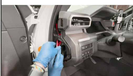
25. With the wires secured, snap the access panel closed.
