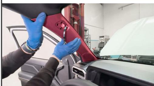
20. Run your cable(s) through your Stealth Pod, and attach it with the supplied bolt and Hex Key.
