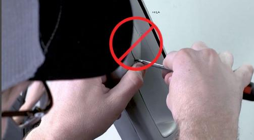
Pinch the small plastic tail on the cap to remove it from the A-Pilar.
