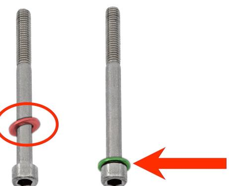
Take care when threading the hex bolt and washer into the Stealth Pod. The washer needs to be flat against the head of the bolt as you thread the bolt in. Otherwise, it will bind and not fully seat.
