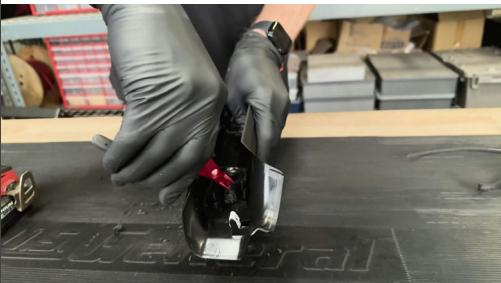
Clean up and plastic burs on the back side with a pair of flush cuts.
