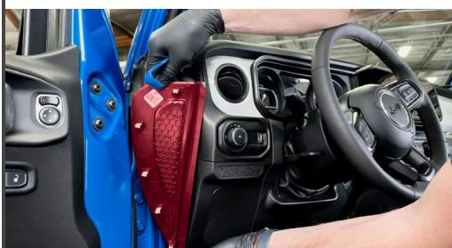
13. Run the Banks OBD-II cable from the bottom and up through to the top of the dashboard.
