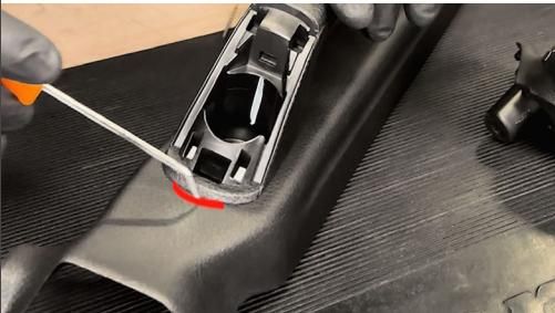
This is to help keep the step bit from walking when drilling. The goal is to avoid damaging the textured portion of the A-Pillar.
