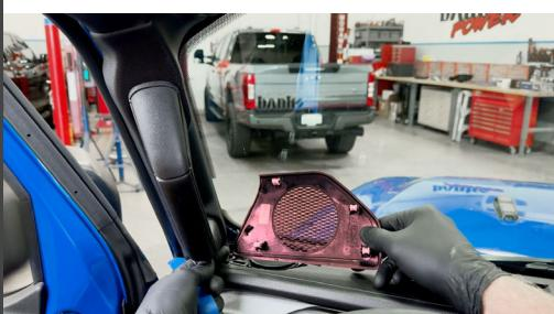
3. With a plastic pry tool, pop off the plastic plugs that cover the A Pillar bolts.
