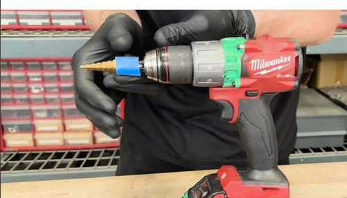
Use a piece of masking tape and mark the appropriate diameter.
