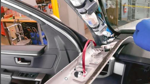
You should be able to fish it through the top area as shown and run the cable through the hole you cut in the pillar.
