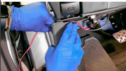
Thread the flat OBD-II Cable through the gap by the kick panel.
