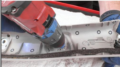
Continue until both sides are drilled to 16-18mm
