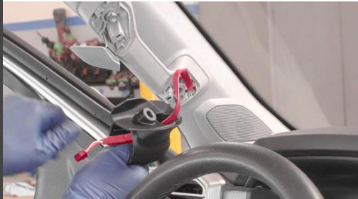
Run the iDash OBD-II cable through the hole on the stealth pod. Thread the supplied Hex Head bolt in, and tighten the pod to the handle with the Hex Key.
