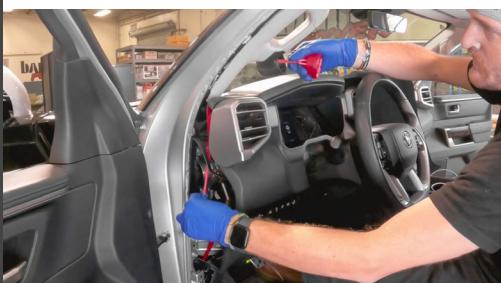
Be sure to leave enough slack on the iDash end to pull the gauge out if needed.
