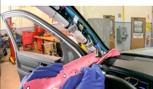
Carefully rotate the pillar to free it from the corner and remove it from the truck. Take care if there is a speaker in the pillar.
