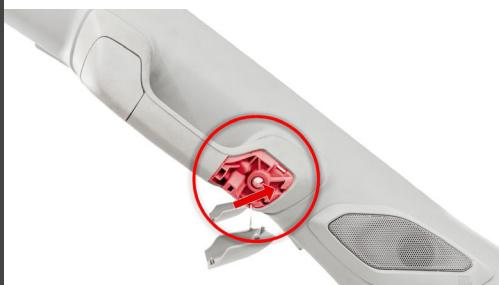
Since this pillar is in two pieces (handle and pillar), you will need to start drilling through both, then remove the handle portion and continue drilling.
