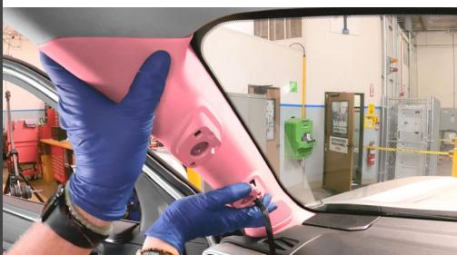
With the corner properly seated, the pillar should snap back into place flush like the passenger side.
