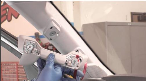
17. Mount the handle back onto the pillar.
