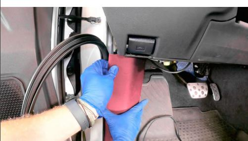
13. Run the iDash Data cable through the side of the dash until it reaches the top. Leaving just enough slack at the bottom to plug the OBD-II end in.
