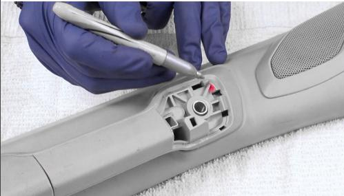
Use a sharpie to mark the corner and try to stay on the inboard side of this corner.
