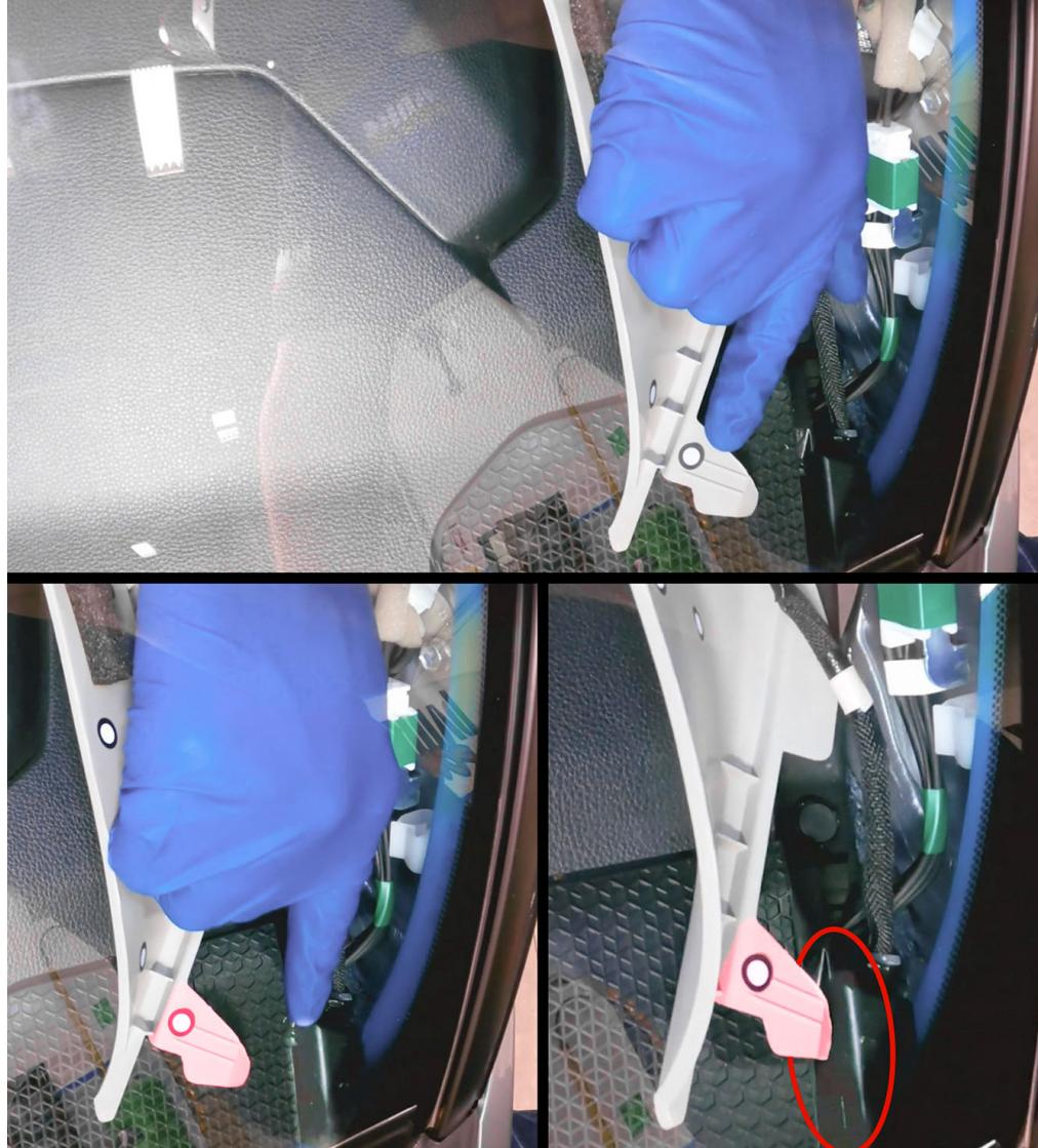
Note: The far end of the pillar has a tab that must go in a hole in the dashboard. If the tab does not slide in, the pillar will not sit flush.
