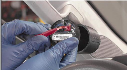
20. Carefully feed the cable back through the pillar and down into the dashboard as you install the iDash into the Stealth Pod.
