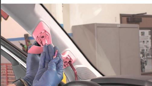
Use the OEM bolt for the top location to hold the handle in place.
