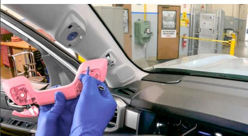
The handle is separate from the pillar and is free to be removed once the bolts are out.
