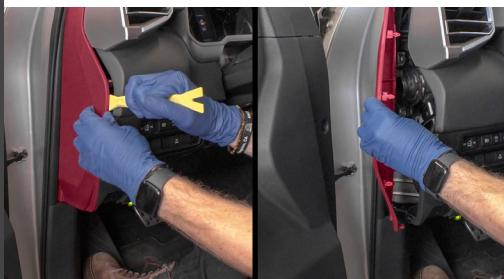
Beware: If you use a screwdriver, it could leave a mark on the soft plastic. A plastic pry tool and/or rag is recommended.
