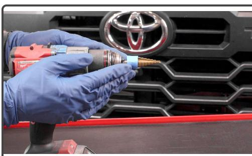
Use masking tape to mark the 18mm location on the step bit.
