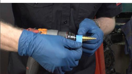
11. Start drilling 90° perpendicular to the spot you marked. Continue to drill until the 2nd or 3rd step.
