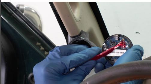
If you have a Derringer or PedalMonster, Plug in the 6 pin connector as well.
