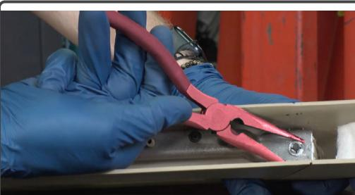
Use a screwdriver or a pair of pliers to keep the washer from spinning.
