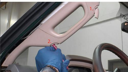
Keep turning the bolt until the handle is free from the truck.
