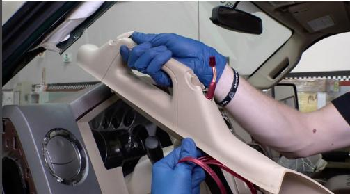
11. Loosely re-attach the A-Pillar. You can thread the top bolt back in a bit by hand to keep the pillar from moving.
