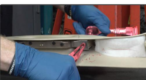
You may need to bend the washer to remove it from the bolt.
