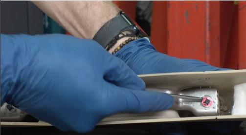
This washer needs to be removed, and will not be reused for the Stealth Pod installation.
