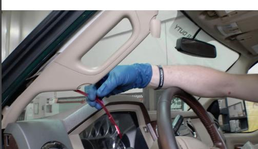
12. Run the cables down the side of the dashboard. Check that you have enough slack in the cable to reach under and into the OBD-II port.
