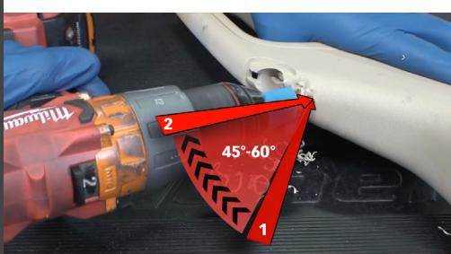
This is to avoid hitting the metal brace and internal plastic on the back side of the pillar.
