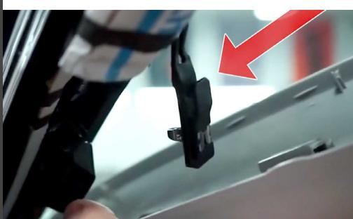
Some trucks have an airbag retainer strap. If your truck does, slide the clip off the plastic trim piece before removing the pillar.
