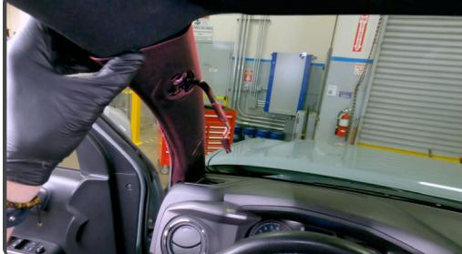
Re-attach and snap the pillar back onto the truck.
