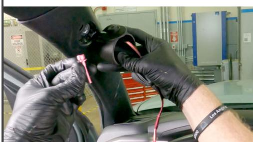
1. Run the cable(s) through the hole you made.
