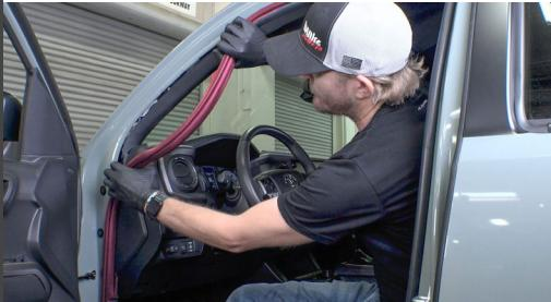
3. Pry off the plastic “SRS” cover that hides the bolt which secures the pillar to the frame.
