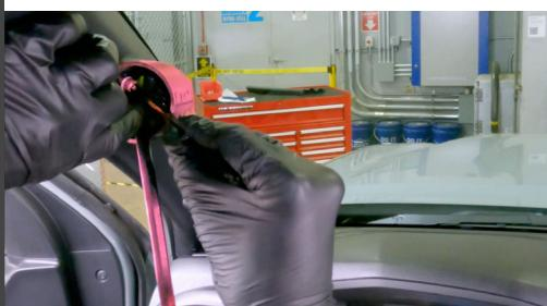
Start by hand and then use the supplied 5mm hex key to tighten it.
