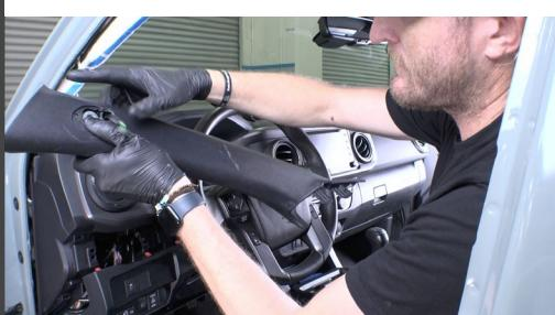
Run the iDash OBD-II cable that you left on your dashboard, through the hole you drilled.
