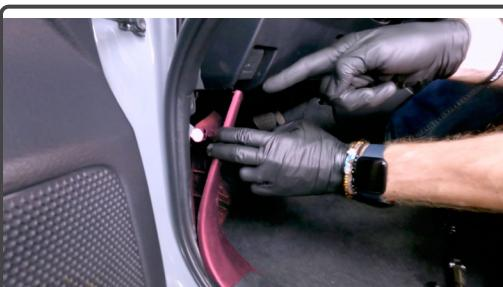
After installing the 3 bolts, re attach the lower left side kick panel as well.
