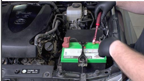
1. Before starting the installation, use your 10mm socket to remove the terminal and disconnect the battery.
