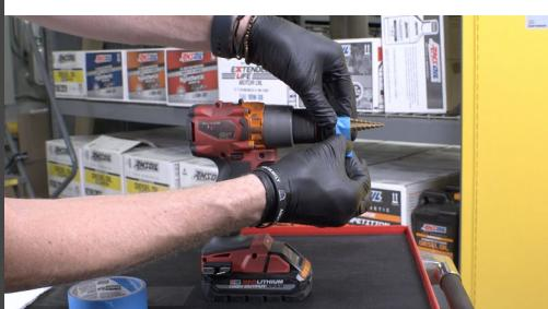
The plastic on the pillar is soft and the drill cuts through it like butter. Use masking tape to mark the 16mm or 18mm mark.
