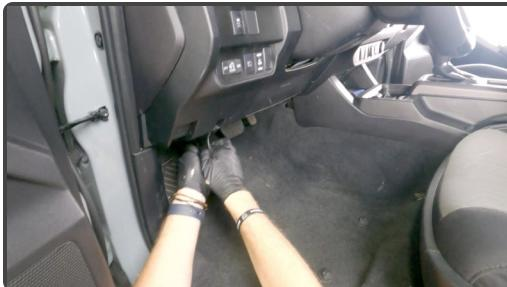
Tidy up the extra OBD-II Cables and tuck it out of the way.
