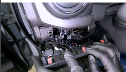
You don't need to fully remove this trim piece, this is just to provide easier access to run your OBD-II cable up through the dash.
