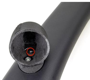
This is how your dot should be when looking through the empty Stealth Pod. Right in the corner of the A-Pillar plastic , and center aligned.
