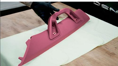
You'll drill a hole near the lower bolt hole, where the cover used to clip in.
