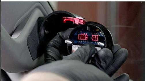
Press the iDash into place, taking care to route the cables back to through the hole and into the pillar as you go.
