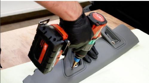
If you have 1 data cable to pass through, drill down to the 16mm step.
