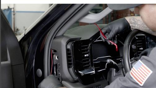
Route the OBD-II cable down through the bottom.
