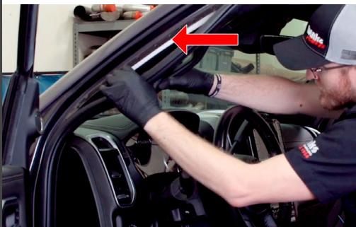
3. Use the plastic pry tool to pry out the small plastic covers that hide the bolts which secure the plastic pillar to the metal frame.
