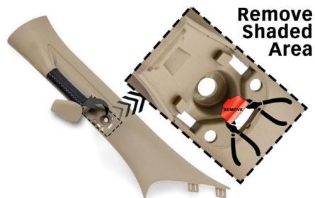
This will allow the iDash data cables to pass through.
