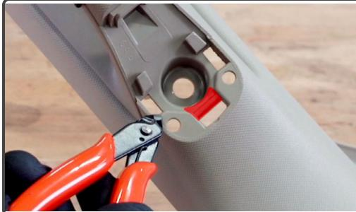
Avoid the sides of the bottom hole since these are used for rigidity. Cut just below the lower bolt hole as highlighted.
