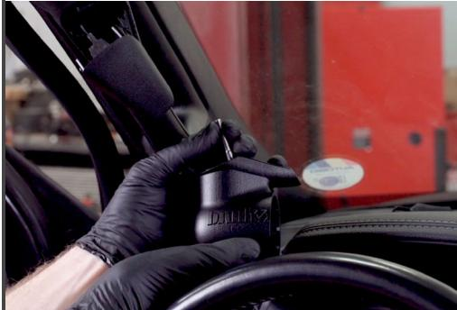
2. Run the cables through the Stealth Pod and then press the Pod flush into the pillar.
