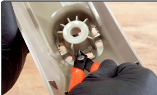
Viewing from the back side, cut halfway down the cylinder, avoiding the sides where the support is.
