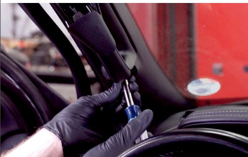
4. With the 10mm socket, remove the two bolts.
