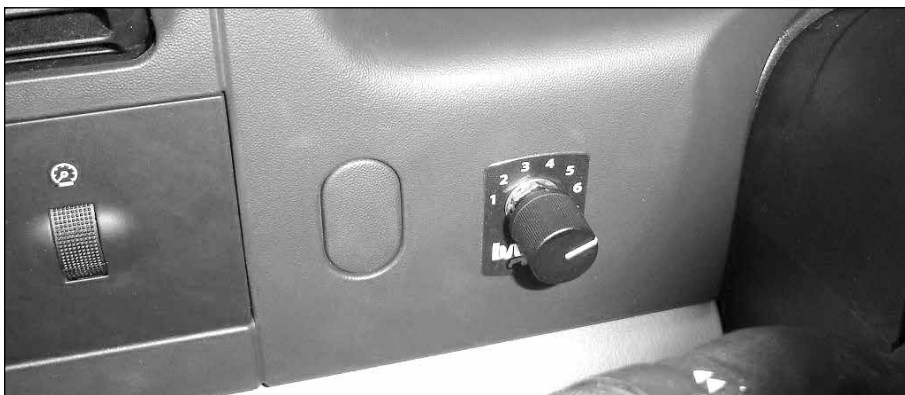
Figure 51: Finished installation of the Power Level Selector Switch on 2005-07 model year vehicles
