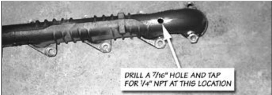
Figure 31: Location to drill and tap the driver side exhaust manifold for the thermocouple
