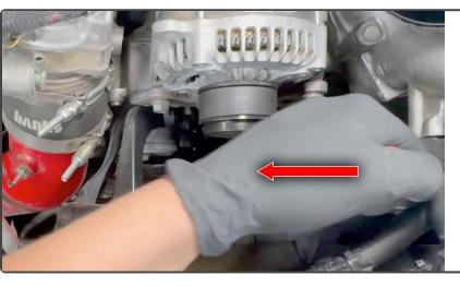
Rotate the ratchet bar counter clockwise towards the passenger side to release tension.
