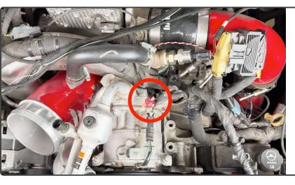
Don't forget the second connection at the rear of the compressor.
