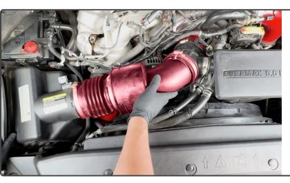
Re-connect the Airbox intake duct.
