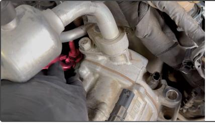
The rear passenger side bolt is. Tricky to get to. It does not have to be fully removed, just back it out enough until the A/C compressor is free.
