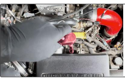
Reinstall the 13mm nut for the resonator.
