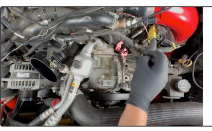
Next, unplug the rear A/C connection and free the harness plastic nuts from the post mount.
