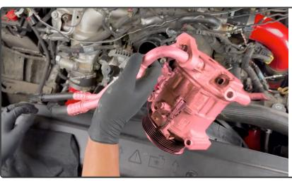
Lift and remove A/C compressor, place it out of the way for now.
