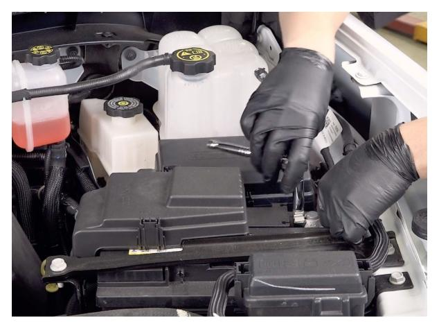
1. With a 10mm socket, loosen and remove the negative terminal on both batteries.
