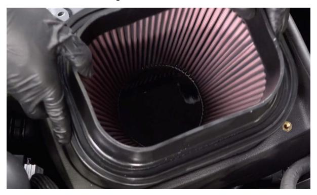
15. Next, install the Banks Big-Ass Air Filter into the Airbox.
