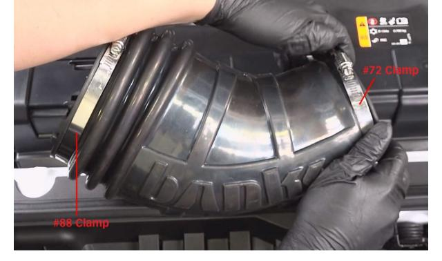
17. Now place the #88 clamp, which is the larger one on the Airbox lid side, and the #72, the smaller clamp on to the turbo side.
