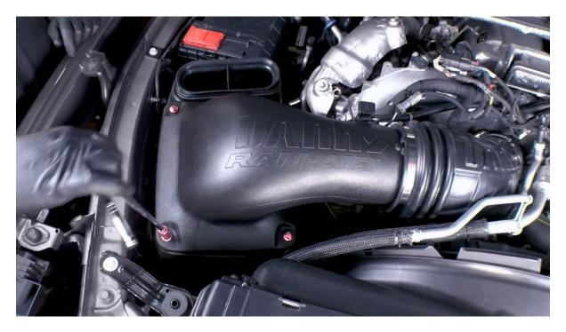
20. Starting with the smallest bolt hole, insert all four, 5/16<sup>th</sup> bolts and hand-tighten. Then use a 10mm socket to snug them but be sure **TO NOT** over tighten.
