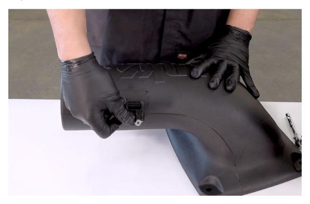
8. Please note that the kit comes with new screws to secure MAF sensor into the Banks Intake Tube.
