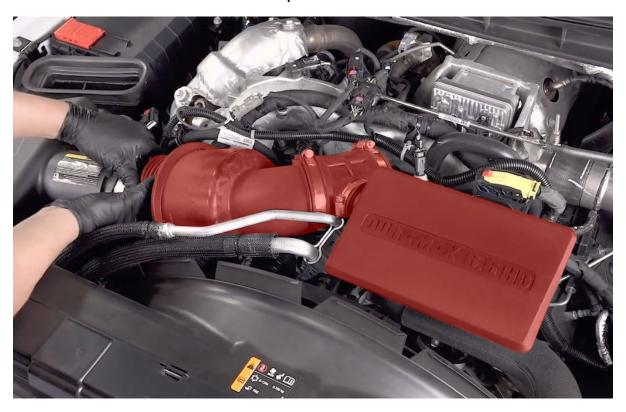
5. Then remove the OEM intake tube.
