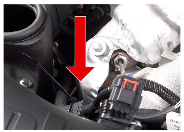
23. With the supplied push mount cable tie, secure the Air Mass Control Module away from any engine components that could get hot.
