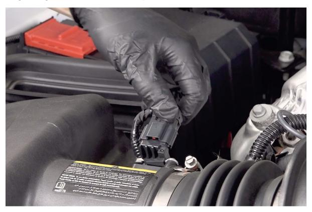
2. To remove the Mass Air Flow Sensor, slide back the red locking tab. Then, press down with your thumb and pull, wiggling gently if necessary.
