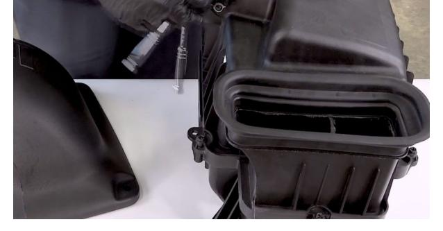
7. Next, remove the Mass Airflow Sensor from the stock airbox using a T20 Torx bit.
