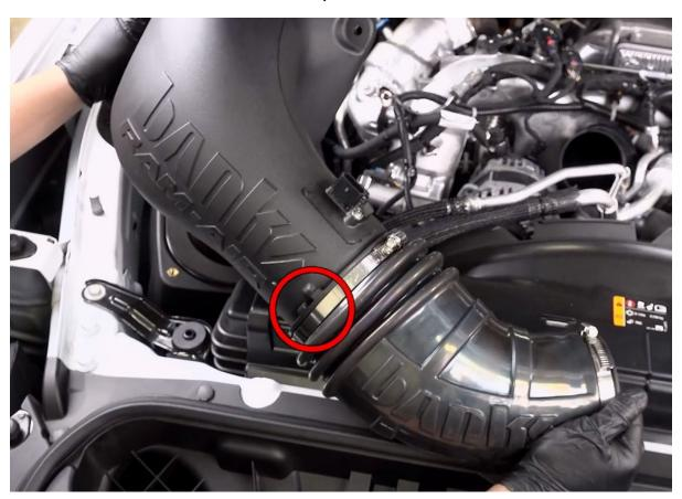
18. Then install the Intake Tube as shown.
