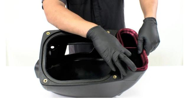
9a. Next, install the Inlet Hood Seal and carefully work the seal into the corners.
