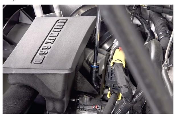
3. With a 13mm socket, remove the nut from the Air Intake Plenum.
