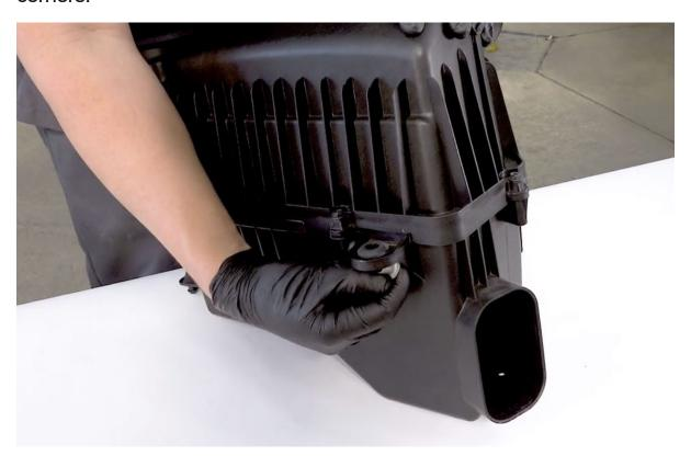
11. Now let's remove the Large Airbox Mounting Grommet from the stock intake.
