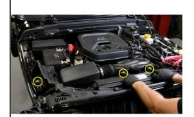
5. Using a 10mm socket, remove the three bolts holding the OEM intake system.
