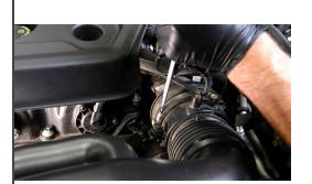
7. Remove the clamp that retains the factory air intake tube to the turbo inlet duct.
