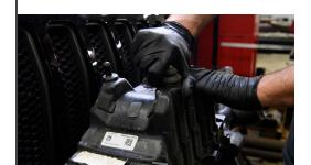
10. Before installing your new Banks Ram-Air kit, remove the rubber grommets from the factory airbox and replace them into the engine bay.
