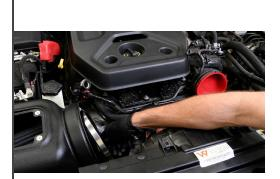
19. Place the larger supplied hose clamp onto the filter.
