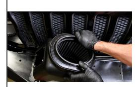
12. Install the Banks air filter into the Banks airbox and make sure the arrow on the filter is on top.
