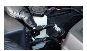
6. Remove the two plastic lines from the air filter housing by pressing the grey tabs and pulling away from the housing.
