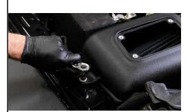
14. Secure the Banks Ram-Air box to the sidewall by using the factory bolt and a 10mm socket.
