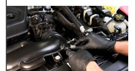
1. Remove the IAT sensor. Pull the locking clip towards you and twist counter-clockwise about 45 degrees until it stops rotating.
