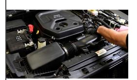
8. Begin removing the assembly by sliding the tube out of the turbo inlet.
