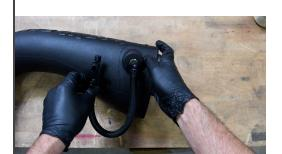
17. Once the fitting is installed, connect the open end of the hose to the fitting. Make sure you can make a loop with the hose, as shown.
