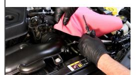
2. Unhook the two clips securing the IAT harness to the factory intake tube. Pull the sensor and harness out of the way. Wrap in a shop towel to avoid any damage to the sensor.
