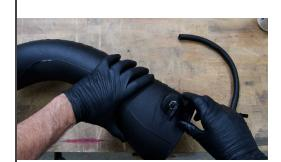
16. Take the supplied plastic barbed hose elbow and thread it into the Banks intake tube. The barbed end should be at the 6 o'clock position.
