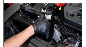
13. Install the Banks Ram-Air box into the engine bay by pressing down until it pops into the rubber grommets.
