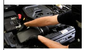
9. Grab the airbox assembly with both hands and pull up until you feel a pop. Pull the assembly out of the engine bay.
