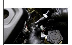
24. Reinstall the two plastic tubes into the vacuum manifold by pushing until you hear a click.
