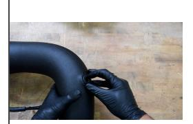
18. Install the rubber grommet for the IAT sensor onto the intake tube.
