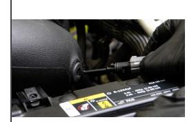
23. Insert the IAT sensor into the rubber grommet.
