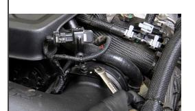
22. Reinstall the vapor pressure sensor bracket with the factory bolts using a 10mm socket.
