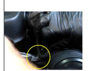
4. Cut off the plastic tie that holds the wiring harness to the OEM intake tube.
