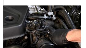
3. Remove the two bolts holding the vapor pressure sensor bracket, using a 10mm socket.
