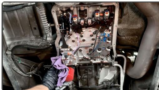
Clean up any excess fluid from the pan mating surface.
