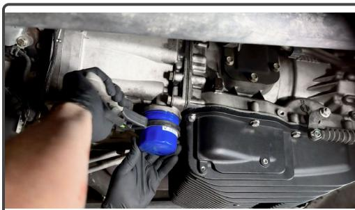
Install new external filter with the magnetic ring pre-installed.
