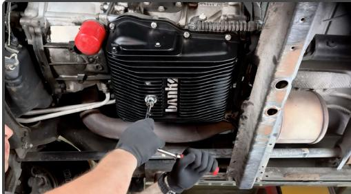
Install the magnetic drain bolt.
