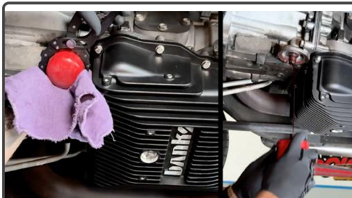
Remove the factory external transmission filter and catch any fluid that leaks out.
