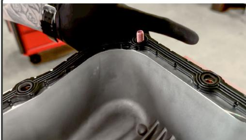
Use a bolt in the corner of the pan to help align the gasket for install.
