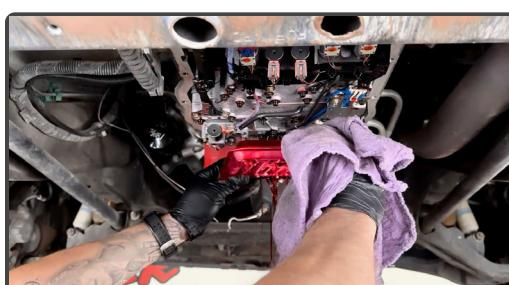
Carefully remove the OE transmission fluid pickup tube & filter.
