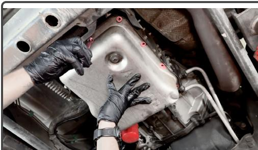
Be sure to support the pan as you remove the bolts to ease removal
