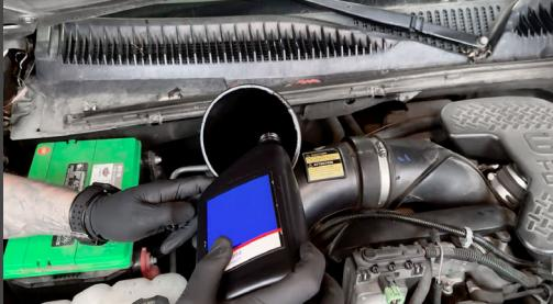
With the vehicle stationary, turn on the truck and run the transmission through each gear position for 5 seconds to pump fresh fluid to all the gear clutch packs.
