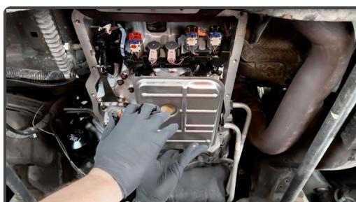
Install new pickup tube into the transmission.
