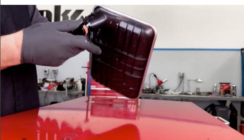
Lubricate the new Transmission Fluid Pickup Tube's rubber seal with transmission fluid.
