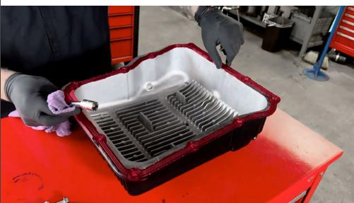
If your original Gasket was in good shape, you can clean and reuse it. Otherwise install a new transmission gasket onto the Ram-Air Pan.
