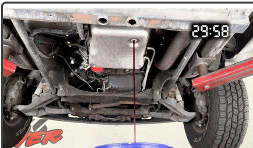
Allow for all the oil to drain from the pan and engine passages. (about 30 min)
