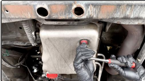
With a XXmm wrench, remove the stock drain bolt.
