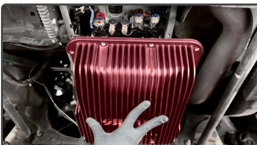
Bring the Ram-Air Pan up to the transmission mating surface.
