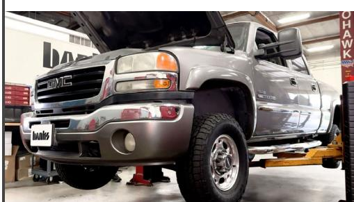
Raise the truck on a lift to provide ample access to the oil pan and the area you will be working with.
