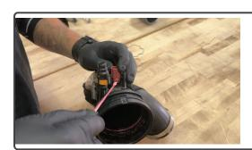
On the cold side boost tube, lift the locking tab on the temperature sensor,
