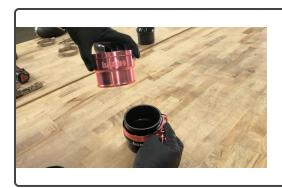
Slide a 4.0" T-bolt clamp over the 3.5" hump hose, and insert the later billet coupler until it fully seats.
