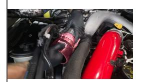
Attach the cold side coupler assembly to the throttle and adjust if the clamp interferes with any stock components or hoses. Be sure the retention clip snaps into place and is secure.
