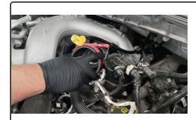
Give the assembly a tug to be sure it is secure, then slip a 4.0″ T-bolt clamp onto the other end.
