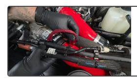
Plug the harness back into the cold side temperature sensor.
