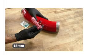
High Output Only: With a 15mm socket, secure the temperature sensor to the hot side boost tube.
