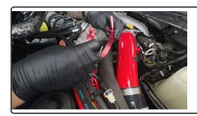
Disassemble a 4.0". T-bolt clamp, and wrap it around the top of the boost tube.
