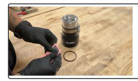
Apply a small dab of the provided silicone lubricant onto the #60 Viton O-Ring.
