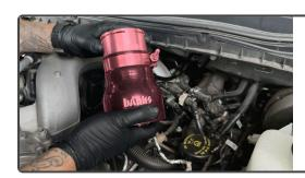
Grab the assembled billet coupler for the compressor outlet.
