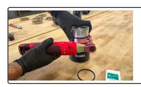
Snug the clamp down. Be sure it's straight and not at an angle or on top of a bead.
