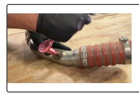
High-Output Only: With a 15mm socket, remove the temperature sensor on the hot side tube.
