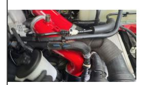
Slip the lower half of the cold side Boost Tube into the reducer elbow. Fully seat the tube until it stops on the internal lip in the elbow.
