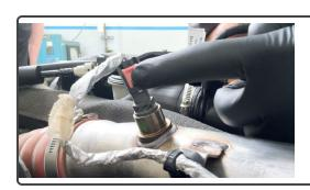
High Output Only: Slide the locking tab up on the hot side temperature sensor.
