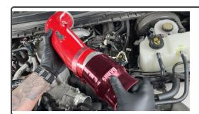
Slip a 4.0" T-bolt clamp and hump hose onto the other end of the Banks Boost Tube.
