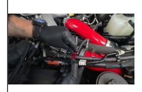
Move the cold side temperature sensor harness clip closer to the driver's side to free up some slack for the sensor.
