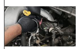
Attach the coupler to the compressor outlet, check that the retaining clip snaps into place, and that the clamp is not rubbing against the intake manifold.
