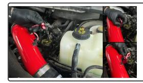
High Output Only: Plug in the Hot-Side temperature sensor and harness.
