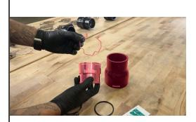
Grab the 3.5" to 2.75" reducer, the smaller of the two billet couplers, and the factory hot side retaining clip removed from the stock coupler.
