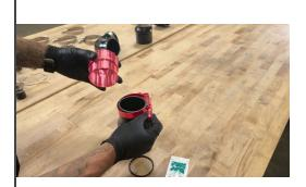
Slip a 3.0" T-bolt clamp onto the reducer, and the billet coupler into the reducer until it fully seats.
