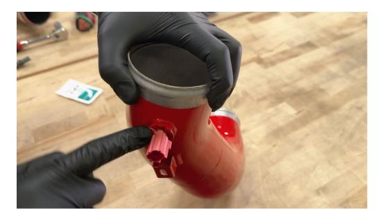
Line the locking tab on the sensor up with the notch on the boost tube.
