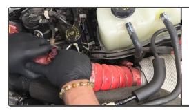
Carefully lift the stock boost tube up and out of the engine bay.
