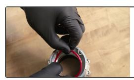
Slide the O-Ring into the groove inside the billet coupler.
