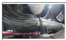
With a long extension, loosen the clamp on the charge air cooler outlet.
