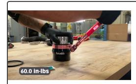
Be sure the clamp is straight and not at an angle or on top of a bead. Torque the clamp to 60 in-lbs
