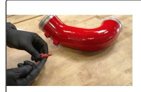
Apply a small amount of the provided silicone lubricant onto the o-ring for the cold side temperature sensor.
