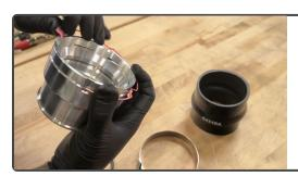
Snap the cold side retaining clip onto the larger billet coupler
