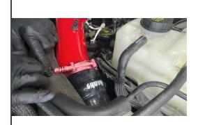
Depending on the year and trim of your Super Duty, you may have to adjust the clamp direction to avoid contact with the stock components.
