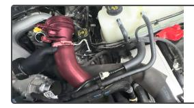
Carefully lift the stock boost tube up and out of the engine bay.
