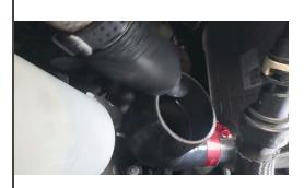
Slip the reducer elbow over the charge air cooler outlet. Leave the clamp loose for now so you can adjust its orientation for the boost tube.
