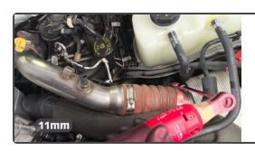
Loosen the clamp on the charge air cooler with an 11mm socket.
