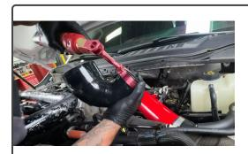
Loosely secure a (3.5" for 2011-2016 or 3.0" for 2017-2025) T-bolt clamp to the end of the reducer elbow.
