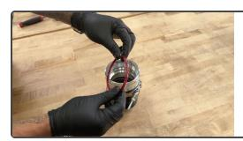
Slide the O-Ring into the groove inside the billet coupler
