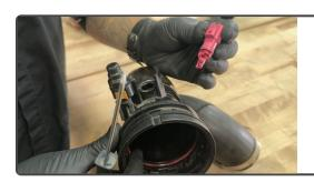
Then twist the sensor to release it from the tube.
