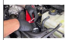
If there is interference, undo the clamp and spin it around so its orientation is not rubbing on any stock components.
