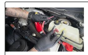
Disassemble the 3.25" T-Bolt clamp so you can wrap it around the Charge Air Cooler inlets hump hose.
