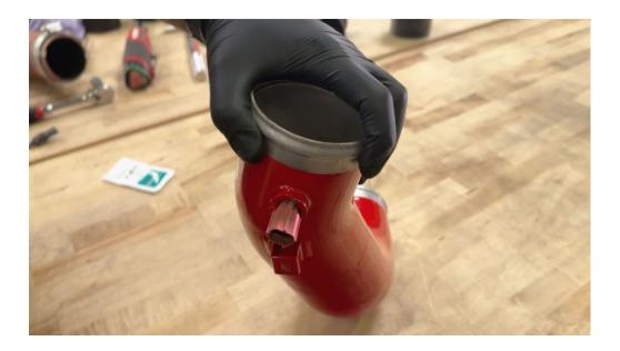
Twist the sensor to lock it; it will snap into place.
