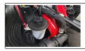
Reinstall the power steering reservoir back to its original location.
