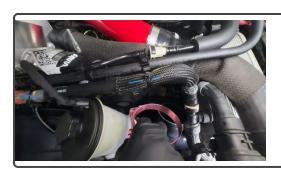
Slip a 4.0" T-bolt clamp over the other end of the reducer elbow.
