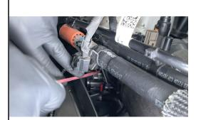
With a flat-head screwdriver, release the retaining clip from the throttle inlet. This factory retaining clip will be transferred to the Banks Cold Side Boost Tube Billet Coupler.
