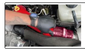
Slide on and fully seat the hump hose onto the charge air cooler inlet.
