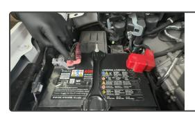
Remove the negative lead from both batteries.
