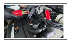
With a 10mm socket, remove the bolt from the power steering reservoir.
