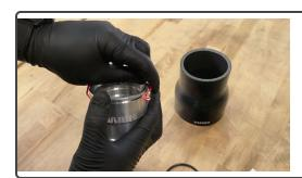
Line the retaining clip up with the groove on the billet coupler; it will snap into place.
