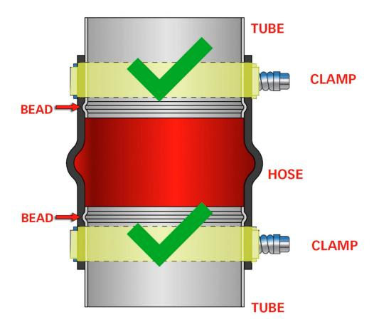
An improper installation, such as a clamp sitting directly on a bead or crossed diagonally, will result in a boost leak.
