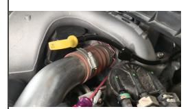
With a flat head screwdriver, pop the retaining clip free from the compressor outlet. This factory retaining clip will be transferred to the Banks Hot Side Boost Tube Billet Coupler. Do not discard this spring clip!
