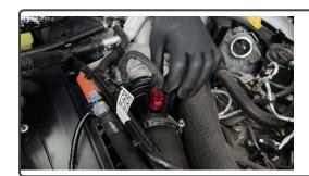
Unplug the temperature sensor on the cold side boost tube.
