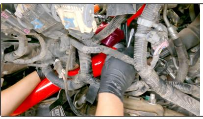
Slip the lower Hot-Side Boost-Tube into the hump hose, and tighten as well.
