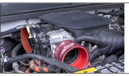
10. Install the upper Cold-Side Boost-Tube Hose (#94312) and Clamps. (#92895 & #92901)
