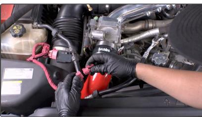
19. Plug in the air intake sensors.
