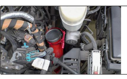
10. Slip on a 4-inch clamp (#92901) on the lower Hot-Side Boost-Tube for now.
