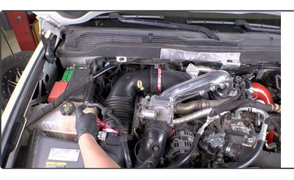
1. Start by loosening the two clamps on the factory intake tube.
