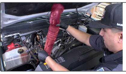
8. Remove the Cold-Side Boost-Tube through the top of the truck.
