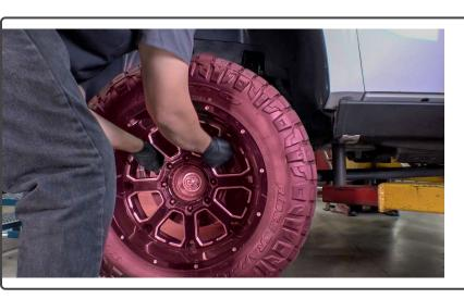
1. Secure the truck on a lift and remove both front wheels to allow for full access.
