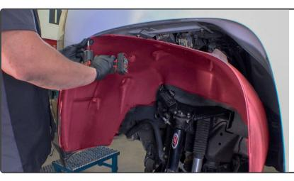
2. Remove both of the front fender liners.
