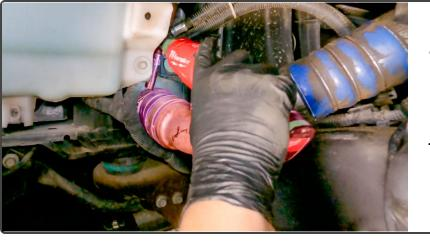
2. Undo the hose clamp holding the bottom of the OEM tube to the charge air cooler Inlet.
