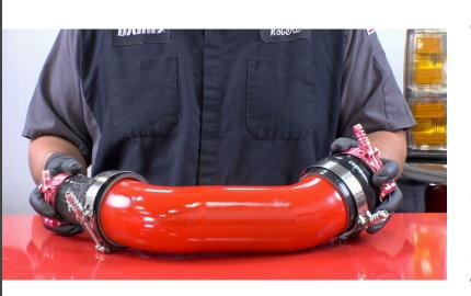
9. Grab the Banks Upper Hot-Side Boost-Tube (#41316), its two hoses (#94299 & #94293), and four clamps. (#92852, and 3x #92901)
