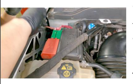
22. Reconnect both batteries. Start the truck and check for any boost leaks or loose clamps.
