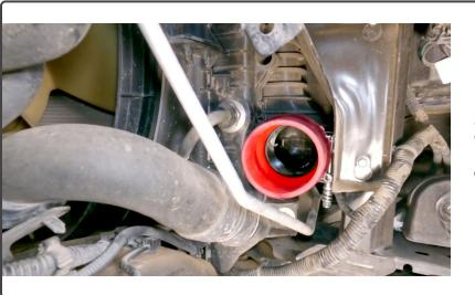
10. Slip the smaller end of the lower cold side hose (#94311) and Clamp (#92897) onto the charge air cooler outlet.
