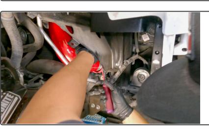
14. Slip the lower hose on, be sure it slides in far enough for the clamp to clear the bead.
