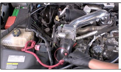
3. Unplug the Air Intake Sensors on the factory air box and cold side boost tube.
