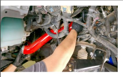
Leave the Boost-Tube loose in the wheel well for now to allow for movement when you install the upper Boost-Tube.
