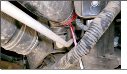
6. Loosen the lower retaining clip of the passenger side boost tube by rotating it counter clockwise.
