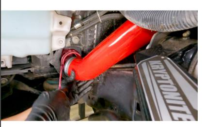
13. Slip the lower hose onto the Boost tube. Be sure it slides in far enough for the clamp to clear the bead. Tighten to 5-ft/lb.
