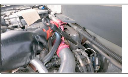
1. Undo the hose clamp holding the top of the OEM hot side tube to the turbo outlet.
