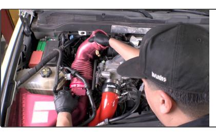
18. Drop in and reinstall the air intake system.
