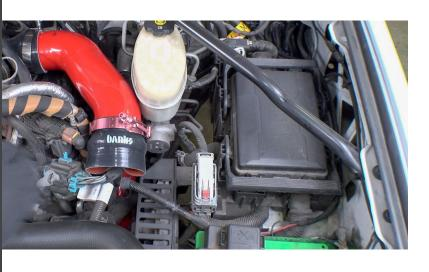
11. Rotate the upper Hot-Side Boost-Tube until the top can slip into the turbo outlet hose.
