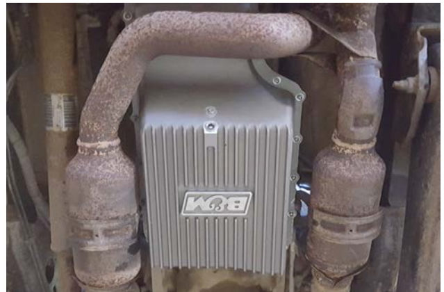
13. Fasten transmission gasket and pan in place using (19 ea.) screws (4) and washers (5) .
