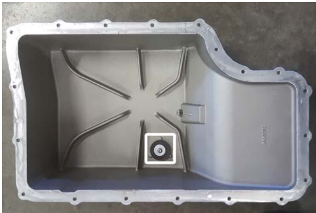
12. Install screw (10) through lock washer (9) , oversized flat washer (12) , and stock magnet (removed at Step 6) then into cast pan.
