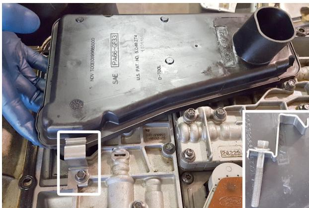
6. Install filter and **clip (9)** onto bolt to secure filter to transmission.
