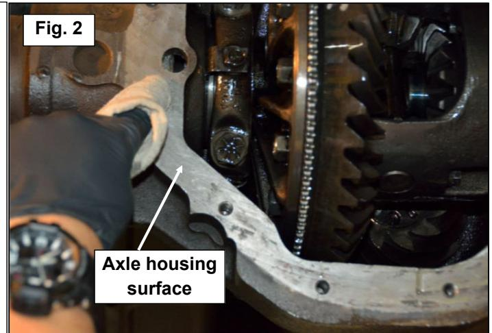
9. We recommend running a 5/16"-18 tap through each threaded cover hole on the axle housing to ensure an accurate torque on all bolts.
