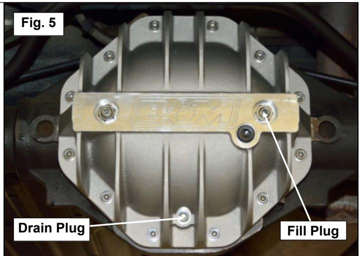
17. Fill with factory recommended gear oil using the B&M Cast Aluminum Rear End Cover fill plug hole (**See Figure 5**). Add gear oil until oil runs out of the B&M Cast Aluminum Rear End Cover fill plug hole.
