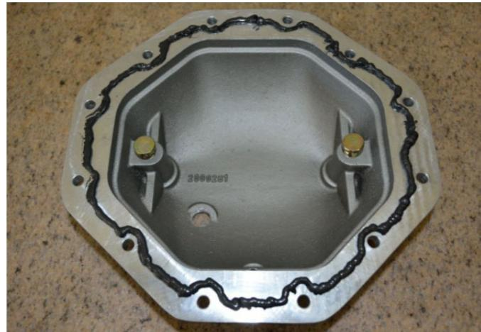
12. Install the cover on the differential housing using the 12 supplied screws and washers. Tighten the screws in an alternating or "criss-cross" pattern to 15 ft-lbs torque.
