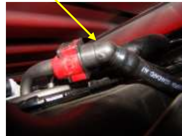
Fuel Tank Suction Tube Figure 13
