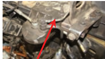
Figure 48 Injector Bleed Line that connects to the tank return line.
