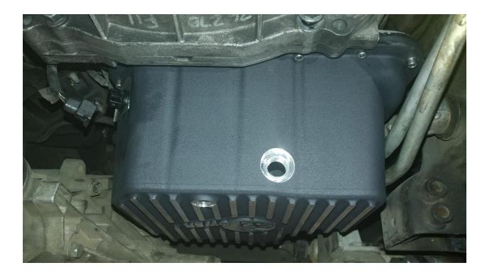
23. Hold the oil pan up into position, aligning the screw holes. Install four (4) M6x1.0x20 socket head screws and M6 flat washers into each of the corners to hold the pan into place.
