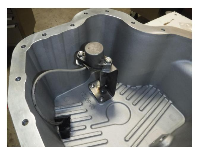
17. Install the sensor to the aFe bracket using the two (2) screws removed in step 15 and the two (2) M6 nuts used in step 9.
