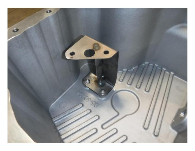
16.Attach the aFe sensor bracket to the aFe oil pan using the two (2) supplied M6x1.0x12 button head screws and M6 flat washers. Make sure the bracket is facing the correct direction as shown above.
