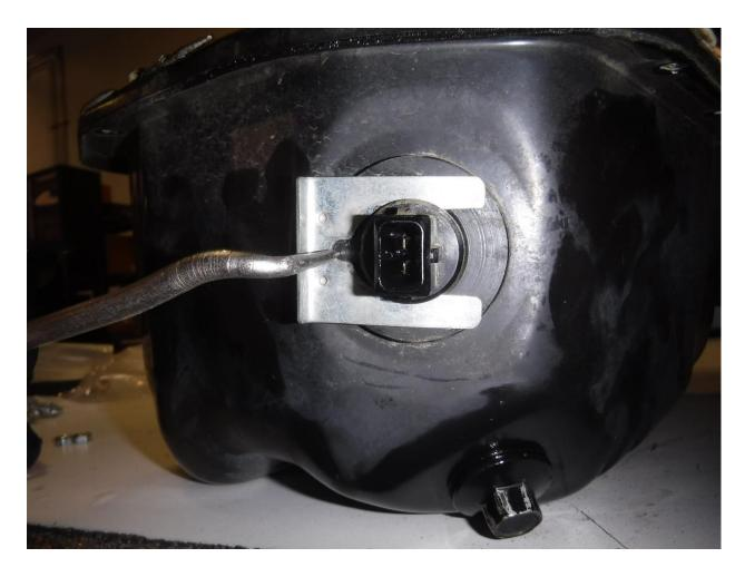
13. Pry the metal holding clip from the outside of the oil pan.
