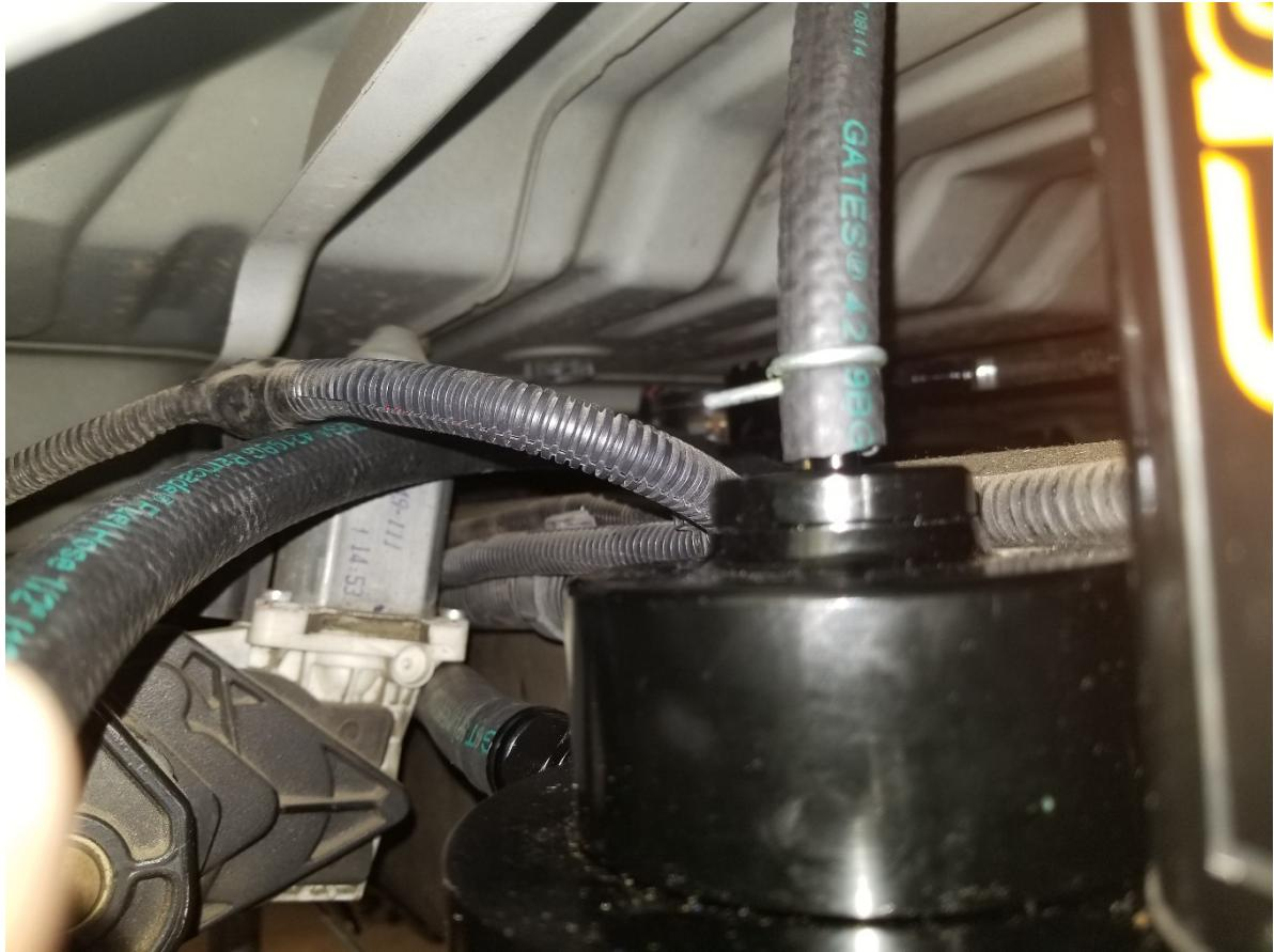
16. Carefully route the  $\frac{1}{4}$ " hose to the top of the air chamber on the fuel manifold assembly, making sure not to kink the hose or allow it near moving parts. Carefully mark and then cut the hose to the correct length. Using the supplied spring clamp, attach the hose to the nipple on the top of the air chamber on the fuel manifold assembly.
