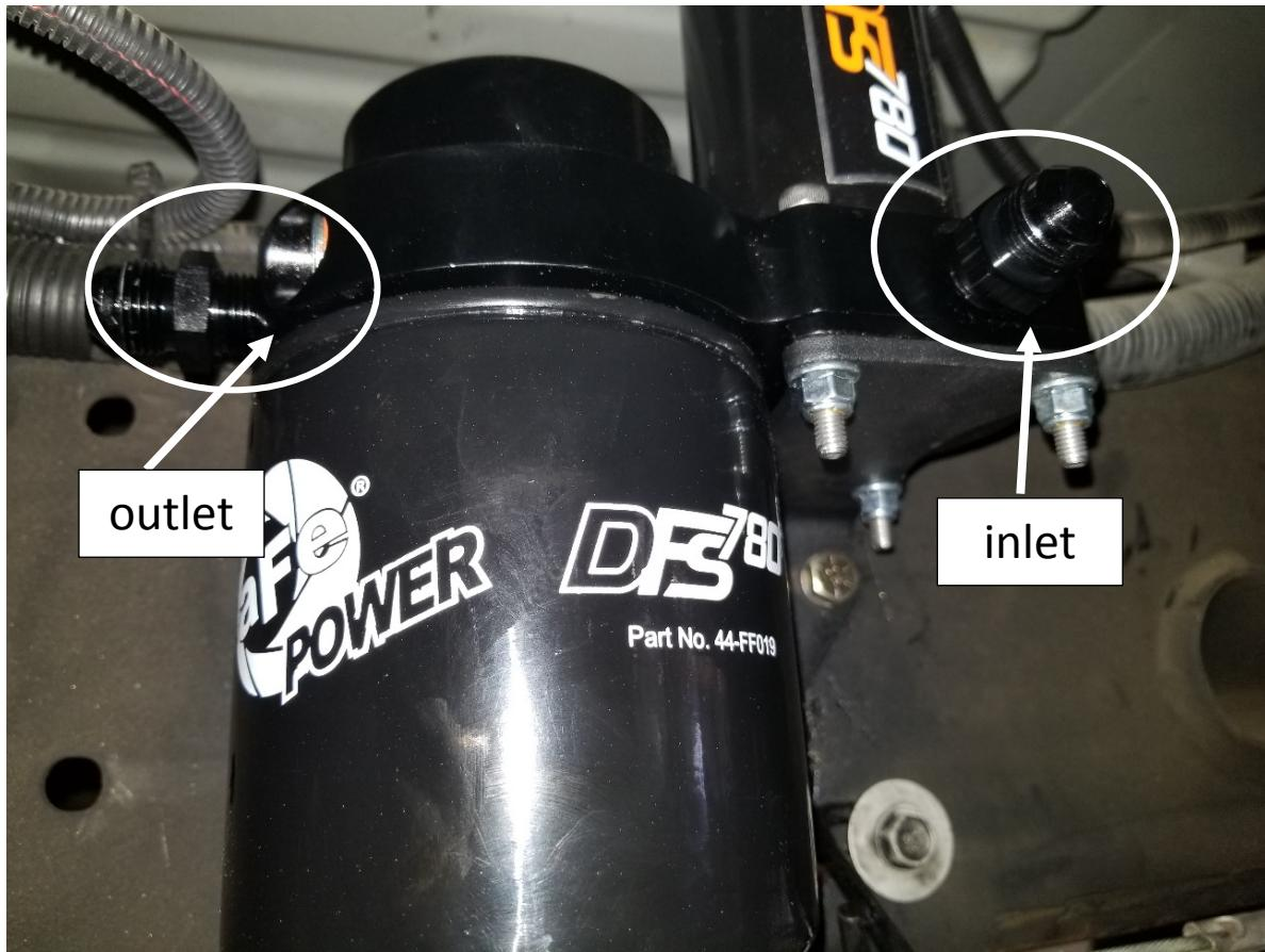
1. Mount the supplied fuel manifold assembly to the supplied carbon steel frame bracket using the supplied hardware and tighten:
