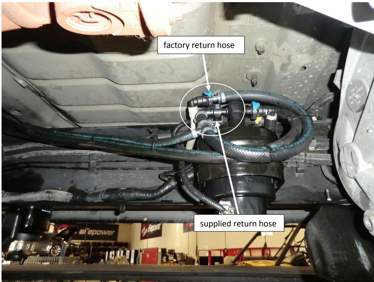
15. Disconnect the factory fuel return line. Attach the supplied fuel return hose between the male and female factory fuel fittings. Push all connections together.
