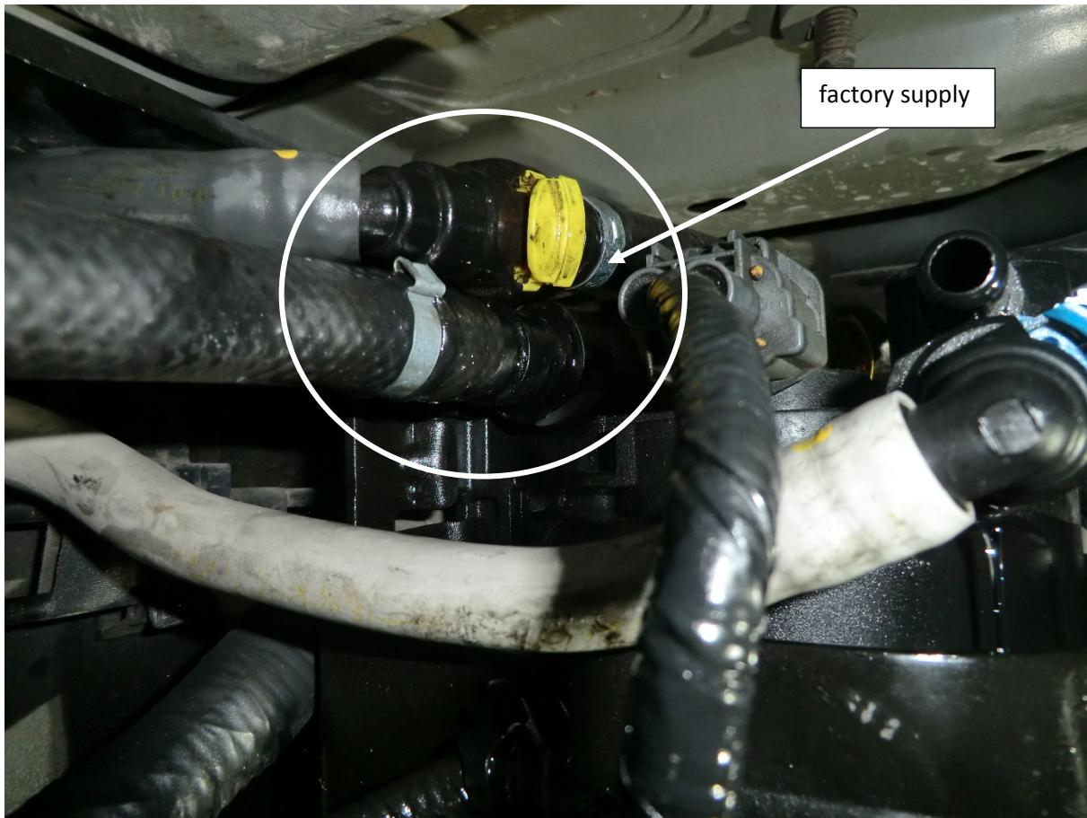
11. Disconnect the factory fuel supply line. Attach the female quick disconnect fitting on the supplied inlet/outlet hose to the factory male quick disconnect fitting on the factory fuel conditioning module. Route the hose to the inlet port on the fuel manifold assembly, making sure not to kink the hose or allow it near moving or hot parts. Carefully mark and then cut the hose to the correct length.
