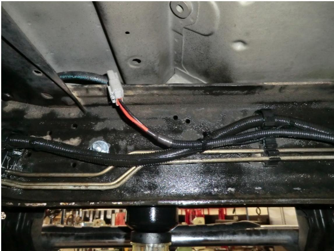
17. Plug the weatherproof connector on the end of the supplied power harness into the mating connector on the fuel manifold assembly motor.
