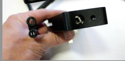
**4.** The billet block installed on the pump itself has a flat knob on the back side that you install the cable into, which is in turn controlled by the knob in the cab. As you turn the knob, the cable will turn the mechanism inside the block and allow the fuel plate a full 2mm of travel.
