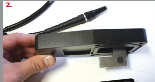
**2.** The heart of the system is the custom machined block with the adjustable fuel plate that gets installed into your P-pump. Using the supplied cable that will be routed into the cab, you'll get full travel of the fuel plate, allowing more or less travel of the fuel rack to control the pump's total fuel output. No more need to pull over, shut the engine off, and slide your plate forward or backward manually anytime you want to adjust your horsepower.
