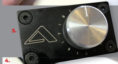
**3.** The custom billet controller is installed inside the cab somewhere on the dash within easy reach of the driver. With 10 clicks on the knob, you have complete control of the pump's output. Lower settings will mean lower fuel output, so better smoke control and fuel mileage, while higher settings allow for more rack travel and maximum fuel output for the drag strip and dyno.
