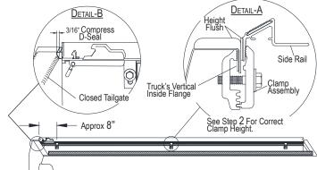
**STEP 2:** For optimum latching performance and cover fit, side rails must be level. To adjust rails, loosen screws and reposition male clamps higher or lower. Tighten all clamps.
