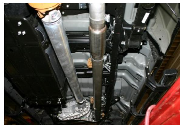
4. Install tailpipes placing metal hangers into OE rubber mounts. Place clamps on all connections.
