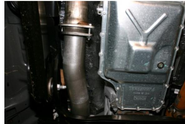
3. Next, install 61113NB pipe, extension pipe (for Crew Cab Long Box) and muffler delete. You can use a stand to support the muffler delete in place.
