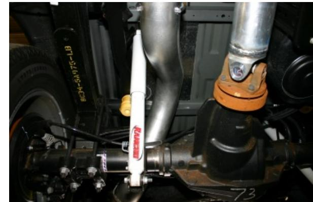
3. Next, install 61152NB pipe, extension pipe (for Crew Cab Long Box) and muffler delete.
