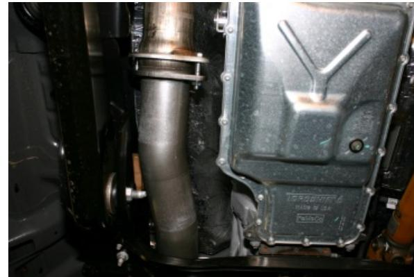
2. Install 61112NB pipe by loosely tightening the flanges together at end of downpipe.
