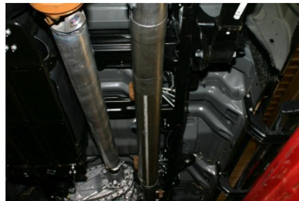
4. Install over the axle pipe and tailpipe placing metal hangers into OE rubber mounts.
