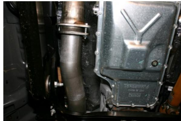
3. Next, install 61152NB pipe, extension pipe (for Crew Cab Long Box) and muffler. You can use a stand to support the muffler in place.
