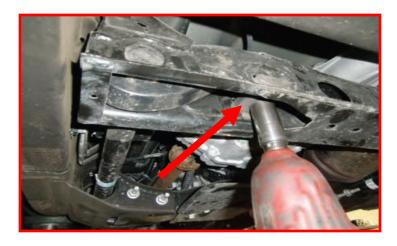
Using a torsion bar unloading tool (ReadyLIFT part #66-7822B), relieve the pressure on the torsion bar cross pin. Take care as the torsion bar is under extreme pressure and can cause injury and/or death if handled improperly. Always use safety equipment.
