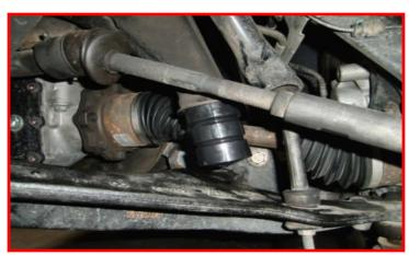
Use the torsion bar unloading tool, load the torsion bar enough to install the cross pin. Remove the torsion bar unloading tool. Install the keyway adjustment bolt using a dab of grease on the threads and tip. This is best to run up until 1/4" threads remain showing between the head of the bolt and the cross pin. This is a starting point for the last steps.
