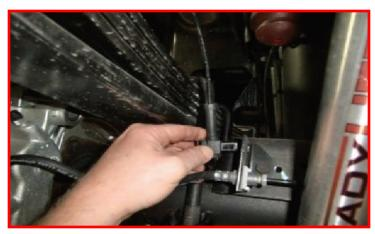
Loosen but do not remove the u-bolts on the passenger side. Remove the u-bolts completely from the driver side.
