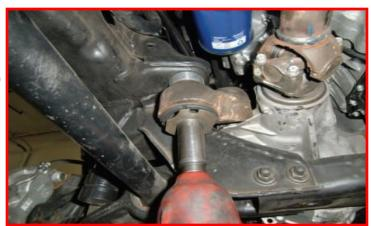
Loosen but do not remove the upper ball joint nut.
