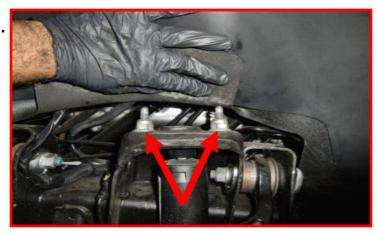
Remove the lower shock hardware. Loosen but do not remove the lower control arm to frame hardware.
