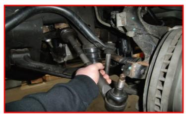
Install the outer tie rod end to the knuckle using the provided hardware. Torque to 65 ft-lbs.
