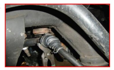
Locate the ReadyLIFT tie rod assembly. Install the provided zerk fittings into the inner and outer tie rod end. There are 2 for the inner.
