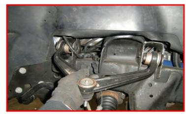
Install the ReadyLIFT upper control arm to the frame using the factory cam bolts and cams. Torque to 125 ft-lbs.
