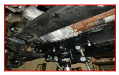
Locate the front and rear differential hanger bolts. Remove all and lower the differential down enough to install the differential spacers.
