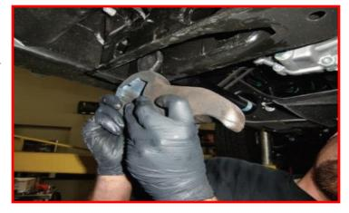
Install the ReadyLIFT keyway into the cross member while sliding the torsion bar into place. The tang of the keyway will be clocked slightly lower than the factory key. This accounts for the lift. Do not load the cross pin or bolt adjuster at this time. This will be done as one of the last steps in the front install.
