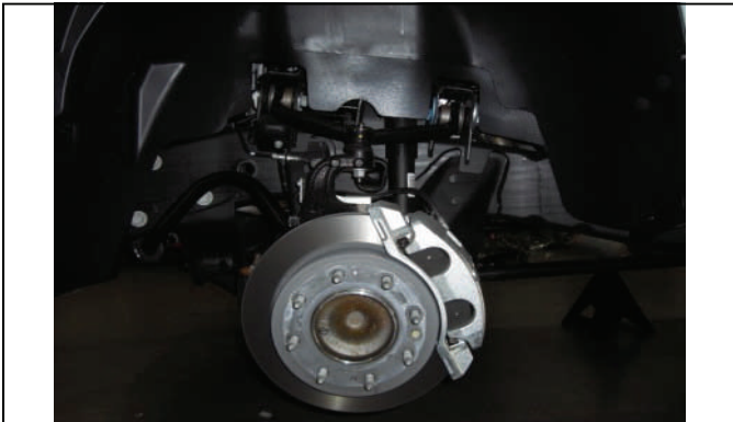
Securely lift vehicle and remove wheels
