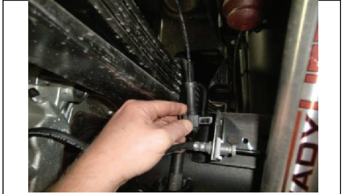
Unhook ABS wire from axle to prevent damage
