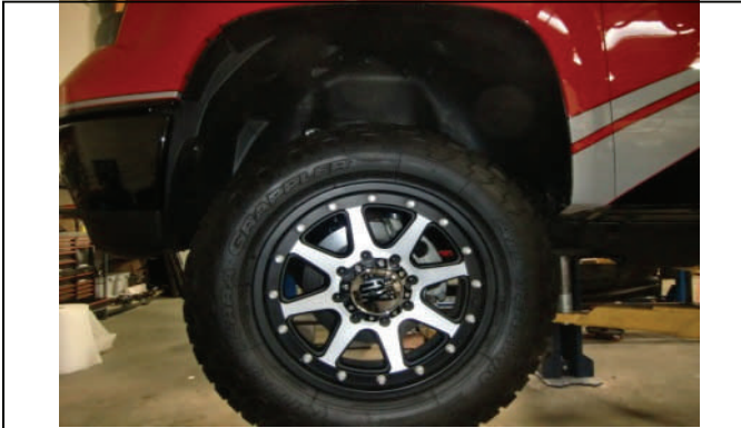
Install wheels/tires lower vehicle to ground check clearances
