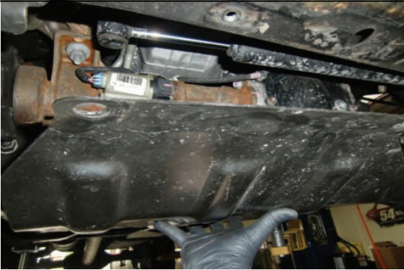
Remove skid plate bolts and skid plate
