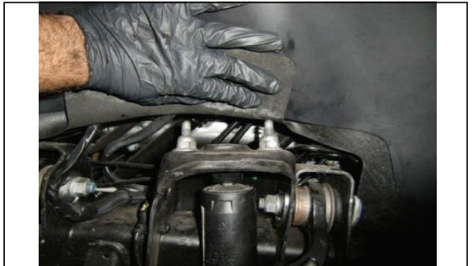
Push back soft fender liner to remove upper shock nuts.
