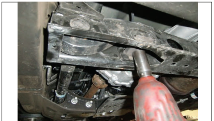
Remove torsion bar adjuster bolt. It will be reused.
