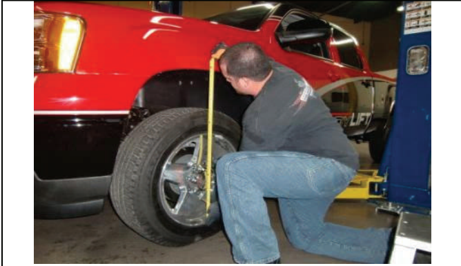
Measure ride height then lift vehicle and remove wheels/tires.
