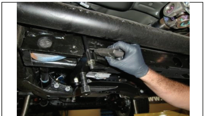
Adjust tool just enough to remove keeper block
