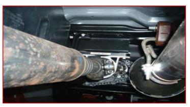
Lower the vehicle to the ground. Torque the lug nuts to the wheel manufacturers specs. Jounce the vehicle a few times to settle to the new ride height. Torque the u-bolts to 110 ft-lbs. Reat-tach the vehicle power source. Have a reputable alignment shop set the alignment to the factory specs.
