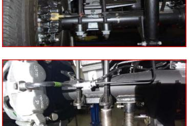
Lower the axle just enough to remove the factory block and install the ReadyLIFT block, making sure not to over extend brake and ABS lines. Adjust as necessary.
