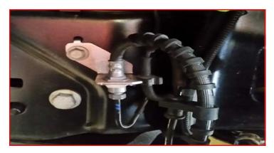
Remove the brake line bracket at the axle.
