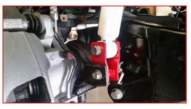
Install the ReadyLIFT brake line bracket to the factory brake line using 5/16" x .75" bolts, washers, and nuts. Install the bolt facing outwards. Gently pull the metal brake line down while lining up the ReadyLIFT bracket to the original holes in the frame. Install using factory hardware. Reattach the brake line bracket at the axle using factory hardware. Torque all to 5 ft-lbs.
