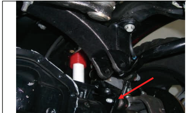
(.05-10) Re-attach and tighten sway bar end links.
