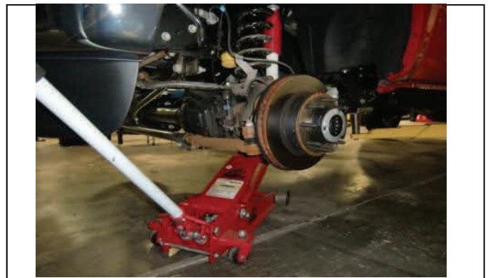
Support front axle with floor jack(s).
