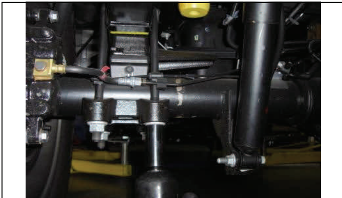
Remove U-bolt nuts and axle mounting plate.
