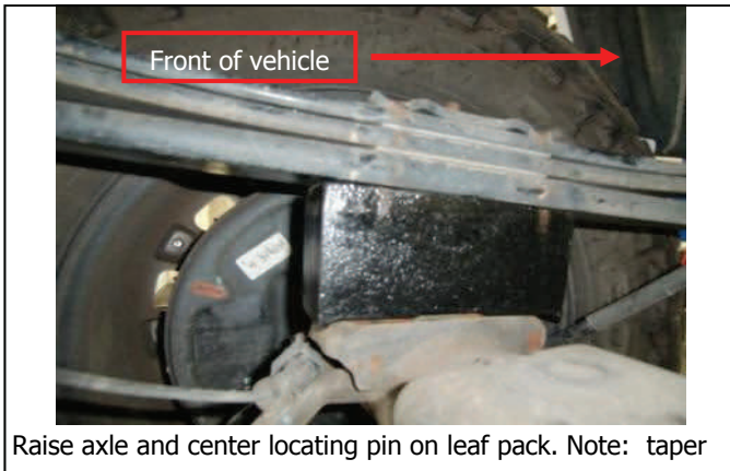
Place new block into position (1.0" block shown)
