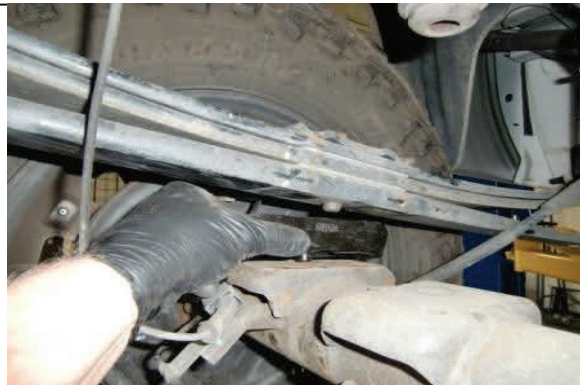
4WD models lower axle and remove factory block
