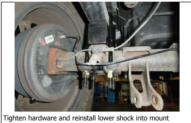
Reinstall axle mounting plate
