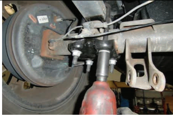
Remove u-bolt mounting hardware
