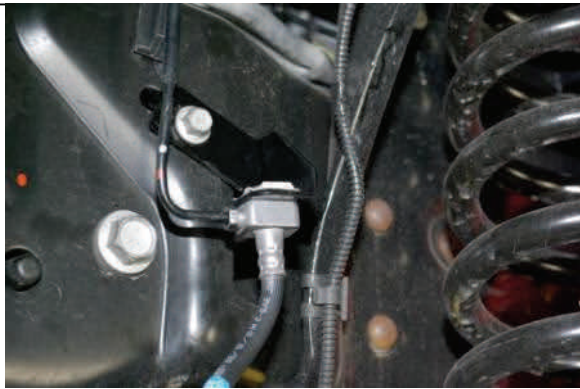
Reinstall block into bracket with retaining clip.
