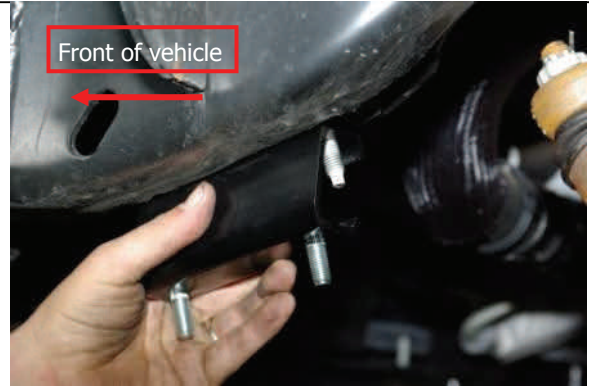
Install provided drop brackets to frame with OE hardware.
