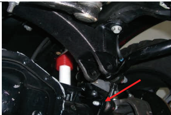
.(05-10) Re-attach and tighten sway bar end links.
