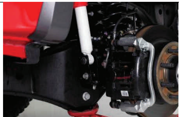
Install and tighten lower shock extension bracket and shock
