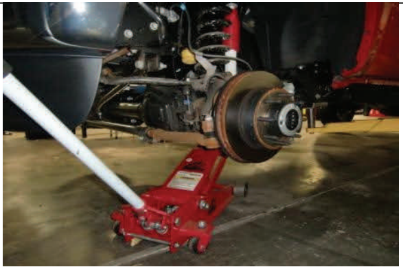
Support front axle with floor jack(s).
